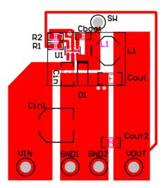
Figure 13. LMR14010A Layout Example
