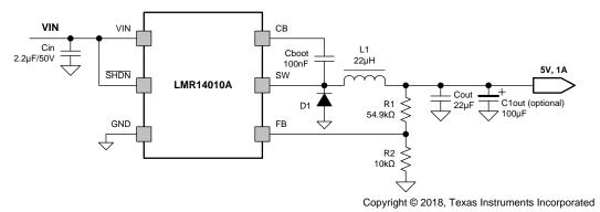
Figure 5. LMR14010A Application Circuit, 5-V Output
