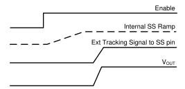
Figure 7-6. Tracking with Shorter Start-up Time than the Internal Ramp
