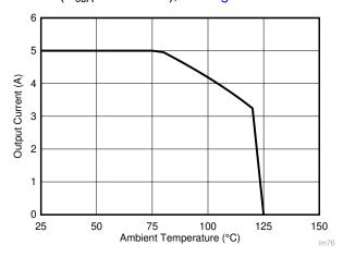
Figure 8-3. LM76005-Q1 Safe Operating Area (5 V<sub>OUT</sub>, 400 kHz, R<sub>0JA</sub>=18.8 °C/W)
