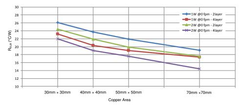
Figure 10-2. Measured R<sub>0JA</sub> versus PCB Copper Area on a 2-Layer Board and a 4-Layer Board
