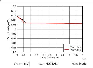
Figure 8-5. LM76005-Q1 Load and Line Regulation
