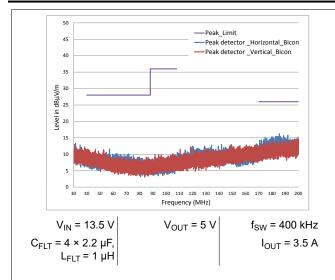
Figure 8-28. LM76005-Q1 Radiated EMI Result vs. CISPR25 Limits - Low Frequency
