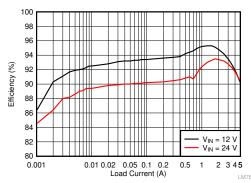
Efficiency: V<sub>OUT</sub> = 5 V, f<sub>SW</sub> = 400 kHz, Auto Mode
