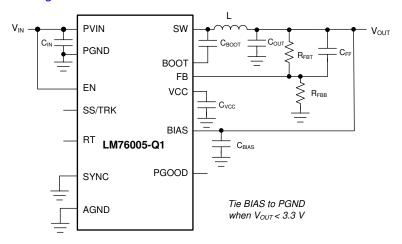
Figure 8-1. LM76005-Q1 Basic Schematic
