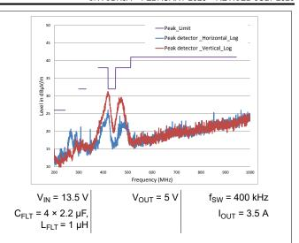
Figure 8-29. LM76005-Q1 Radiated EMI Result vs. CISPR25 Limits - High Frequency
