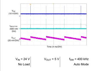
Figure 8-8. LM76005-Q1 Switching Waveform and Output Ripple
