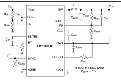
Figure 8-2. LM76005-Q1 Comprehensive Schematic
