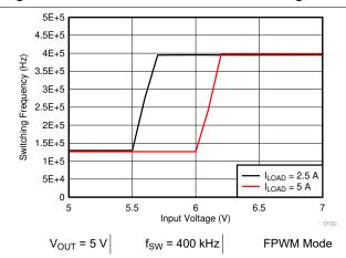
Figure 8-6. LM76005-Q1 Voltage Dropout
