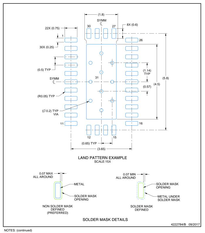
4. This package is designed to be soldered to a thermal pad on the board. For more information, see Texas Instruments literature number SLUA271 (www.ti.com/lit/slua271).
