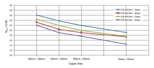
Figure 90. Measured  $R_{\theta JA}$  vs PCB Copper Area on a 2-Layer Board and a 4-Layer Board
