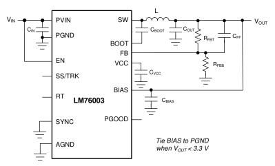
Figure 21. LM76002-Q1/LM76003-Q1 Basic Schematic
