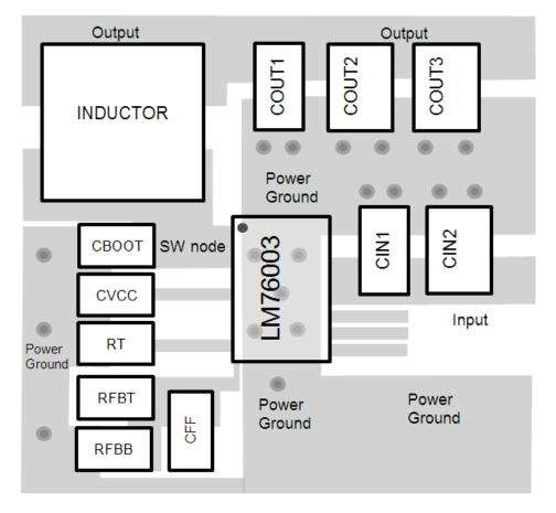
Figure 91. LM76002-Q1/LM76003-Q1 Layout
