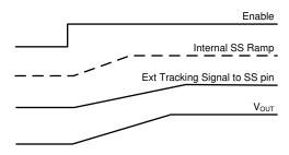
Figure 15. Tracking With Longer Start-up Time Than The Internal Ramp
