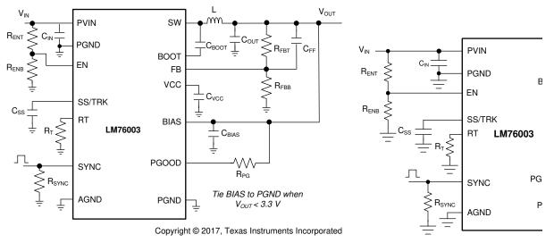
Figure 22. LM76002-Q1/LM76003-Q1 Comprehensive Schematic
