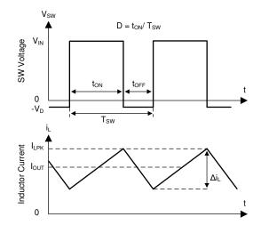
Figure 10. SW Node and Inductor Current Waveforms in Continuous Conduction Mode
