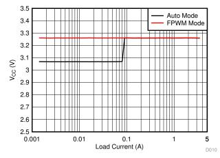
Figure 13. V<sub>CC</sub> Voltage Change With Mode Change
