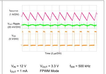
Figure 9-45. LM73606-Q1 Switching Waveform and V<sub>OUT</sub> Ripple
