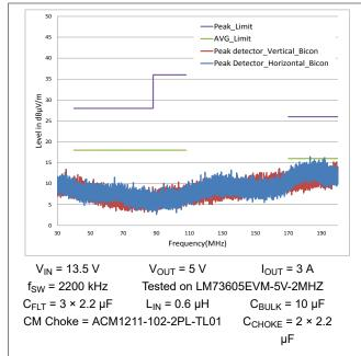
Figure 9-69. LM73606-Q1 Radiated EMI Result versus CISPR25 Limits - Low Frequency
