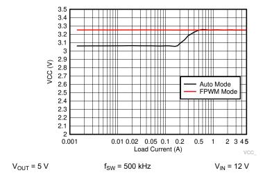
Figure 8-8. VCC Voltage versus Load Current
