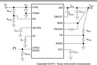
Figure 9-2. LM73605-Q1/6-Q1 Comprehensive Schematic with All Features Utilized
