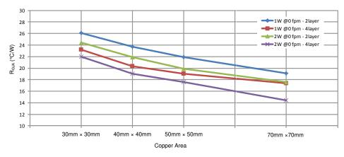
Figure 9-2. Measured R<sub>9JA</sub> versus PCB Copper Area on 2-Layer Boards and 4-Layer Boards
