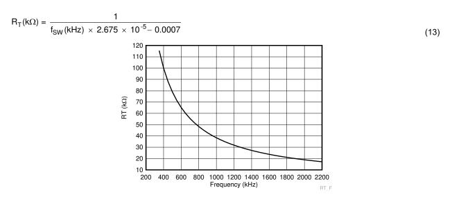
Figure 8-12. R<sub>T</sub> Resistance versus Switching Frequency
