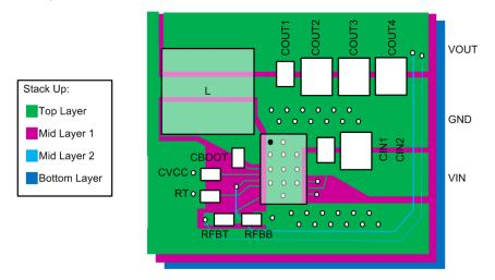
Figure 9-3. LM73605-Q1/6-Q1 Layout Example
