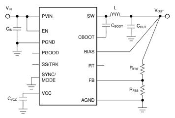
Figure 9-1. LM73605-Q1/6-Q1 Basic Schematic
