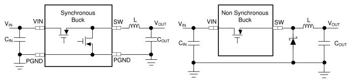
Figure 8-1. Simplified Synchronous versus Non-synchronous Buck Converters
