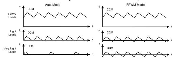
Figure 8-2. Inductor Current Waveforms at Auto Mode and FPWM Mode with Different Loads
