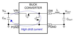
Figure 9-1. Pulsing Current Path of Buck Converter
