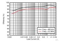
Efficiency versus Load Current V<sub>OUT</sub> = 5 V, V<sub>IN</sub> = 12 V. Auto Mode
