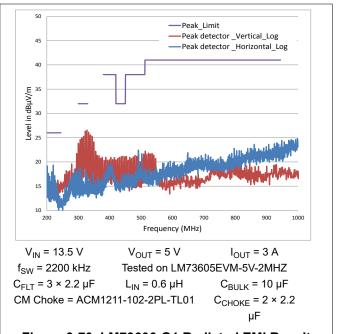
Figure 9-70. LM73606-Q1 Radiated EMI Result versus CISPR25 Limits - High Frequency
