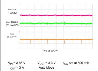
Figure 9-50. LM73606-Q1 Switching Waveform at **Dropout**
