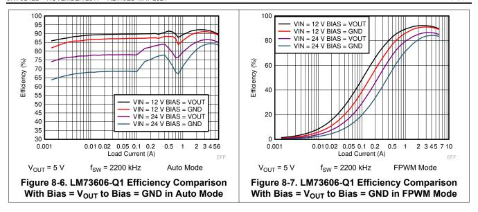
TI recommends tying the BIAS pin to  $V_{OUT}$  when  $V_{OUT}$  is equal to or greater than 3.3 V and no greater than 18 V. Tie the BIAS pin to ground when not in use. A ceramic capacitor,  $C_{BIAS}$ , can be used from the BIAS pin to ground for bypassing. If  $V_{OUT}$  has high frequency noise or spikes during transients or fault conditions, a resistor (1 to 10  $\Omega$ ) connected between  $V_{OUT}$  to BIAS can be used together with  $C_{BIAS}$  for filtering.
