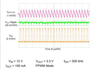
Figure 9-47. LM73606-Q1 Switching Waveform and V<sub>OUT</sub> Ripple
