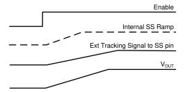
Figure 8-10. Tracking With Longer Start-up Time Than the Internal Ramp
