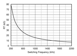
Figure 8-1. Switching Frequency versus R<sub>T</sub>
