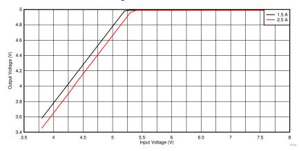
Figure 8-9. Overall Dropout Characteristic V<sub>OUT</sub> = 5 V, Refer to LM63615/25 Data Sheet
