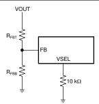
Figure 9-2. Feedback Divider for Adjustable Output Voltage Setting
