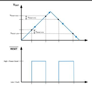
Figure 8-3. Static RESET Operation
