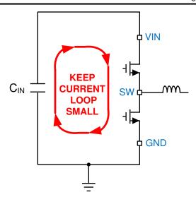
Figure 11-1. Current Loops With Fast Edges
