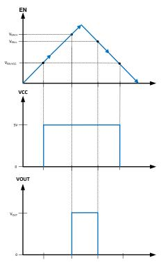
Figure 8-2. Precision Enable Behavior
