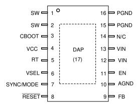
Figure 6-1. PWP Package 16-Pin HTSSOP With PowerPAD Top View
