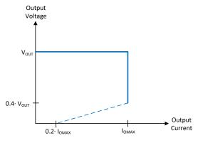
Figure 8-12. Output Voltage versus Output Current in Current Limit
