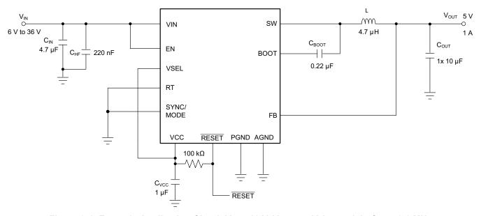
Figure 9-1. Example Application Circuit  $V_{IN}$  = 12 V,  $V_{OUT}$  = 5 V,  $I_{OUT}$  = 1 A,  $f_{SW}$  = 2.1 MHz
