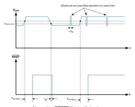
Figure 8-4. RESET Timing Behavior
