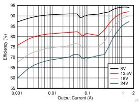
Typical Efficiency At 5-V Vout, 2.1 MHz
