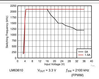
Figure 9-11. Switching Frequency versus Output
