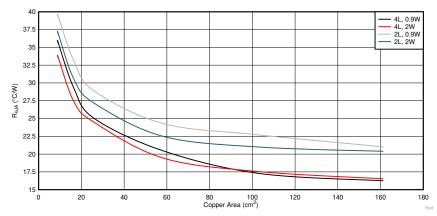
Figure 9-4. Typical R<sub>0JA</sub> versus Copper Area for the HTSSOP Package
