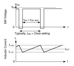
Figure 8-18. Current Limit Waveforms
