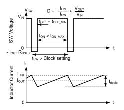
Switching waveforms while in dropout. Inductor current takes longer than a normal clock to reach the desired peak value. As a result, frequency drops. This frequency drop is limited by  $t_{ON\_MAX}$ .
