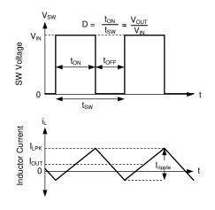
In FPWM mode, Continuous Conduction (CCM) is possible even if I<sub>OUT</sub> is less than half of I<sub>ripple</sub>.
