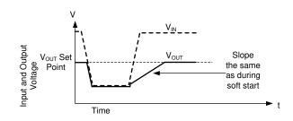
Whether output voltage falls due to high load or low input voltage, once the condition that causes output to fall below its set point is removed, the output climbs at the same speed as during start-up. Even though hiccup does not trigger due to dropout, it can, in principle, be triggered during recovery if output voltage is below 0.4 times the output set point for more than 128 clock cycles.
