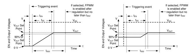
Soft start works with both output voltages starting from 0 V on the left curves, or if there is already voltage on the output, as shown on right. In either case, output voltage must reach within 10% of the desired value  $t_{SS}$  after soft start is initiated. During soft start, FPWM and hiccup are disabled. Both hiccup and FPWM are enabled once output reaches regulation or  $t_{SS2}$ , whichever happens first.
