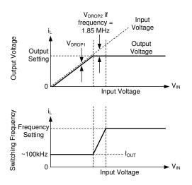
Output voltage and frequency versus input voltage: If there is little difference between input voltage and output voltage setting, the IC reduces frequency to maintain regulation. If input voltage is too low to provide the desired output voltage at approximately 110 kHz, input voltage tracks output voltage.
