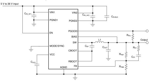
Figure 9-1. Example Application Circuit
