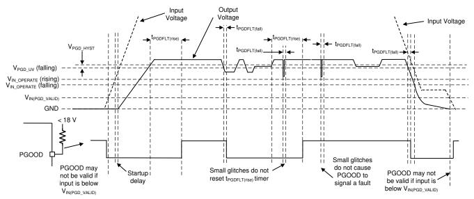
Figure 8-13. PGOOD Timing Diagram (Excludes OV Events)
