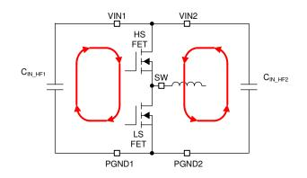
Figure 11-1. Input Current Loop
