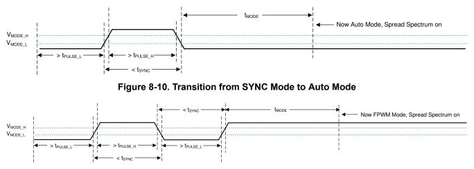
Figure 8-11. Transition from SYNC Mode to FPWM Mode
