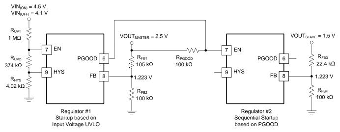
Figure 45. Master-Slave Sequencing Implementation Using PGOOD and EN
