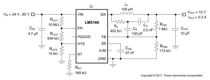
Figure 84. Schematic for Design 5 With  $V_{OUT} = 12 \text{ V}$ ,  $I_{OUT(max)} = 300 \text{ mA}$ ,  $F_{SW(nom)} = 400 \text{ kHz}$
