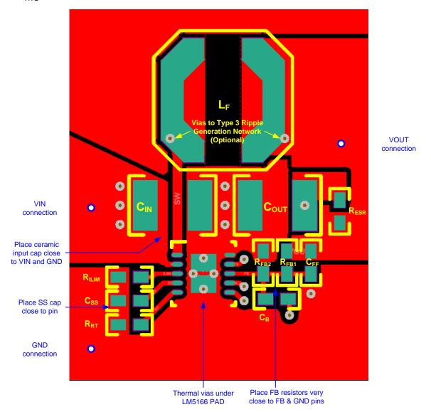
Figure 90. LM5166 Single-Sided PCB Layout Example
