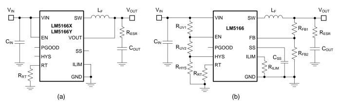
Figure 40. COT Mode Converter Schematics: (a) Fixed Output Voltage of 5 V or 3.3 V, (b) Adjustable Output Voltage With Programmable Soft Start, Current Limit, and UVLO
