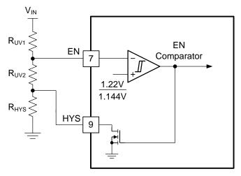
Figure 44. Input Voltage UVLO Using EN and HYS
