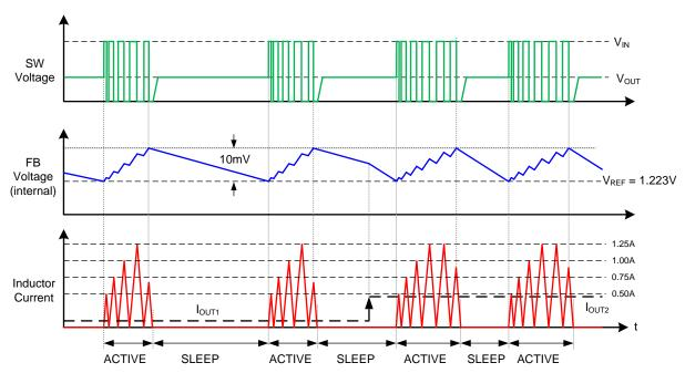
Figure 42. PFM Mode With Modulated I<sub>LIM</sub>, Output Voltage and Inductor Current Representative Waveforms
