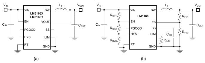
Figure 39. PFM Mode Converter Schematics: (a) Fixed Output Voltage of 5 V or 3.3 V, (b) Adjustable Output Voltage With Programmable Soft Start, Current Limit, and UVLO
