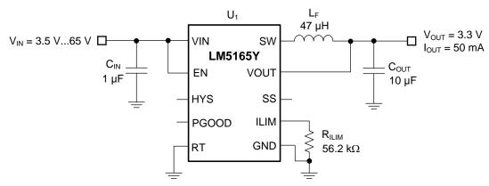
Figure 50. Schematic for Design 2 With  $V_{IN(nom)} = 12 \text{ V}$ ,  $V_{OUT} = 3.3 \text{ V}$ ,  $I_{OUT(max)} = 50 \text{ mA}$ ,  $F_{SW(nom)} = 350 \text{ kHz}$
