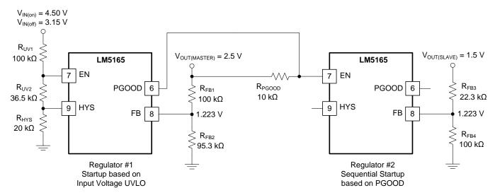
Figure 36. Master-Slave Sequencing Implementation Using PGOOD and EN
