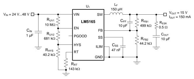
Figure 65. Schematic for Design 5 With  $V_{IN(nom)} = 36 \text{ V}$ ,  $V_{OUT} = 15 \text{ V}$ ,  $I_{OUT(max)} = 150 \text{ mA}$ ,  $F_{SW(nom)} = 600 \text{ kHz}$
