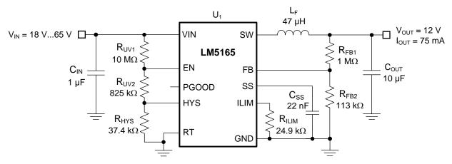
Figure 57. Schematic for Design 3 With  $V_{IN(nom)} = 24 \text{ V}$ ,  $V_{OUT} = 12 \text{ V}$ ,  $I_{OUT(max)} = 75 \text{ mA}$ ,  $F_{SW(nom)} = 500 \text{ kHz}$
