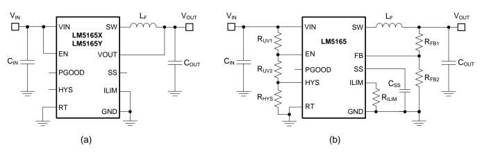
Figure 31. PFM Mode Converter Schematics: (a) Fixed Output Voltage of 5 V or 3.3 V, (b) Adjustable Output Voltage With Programmable Soft Start, Current Limit, and UVLO
