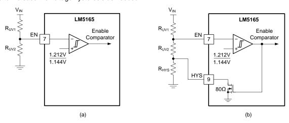
Figure 35. Programmable Input Voltage UVLO With (a) Fixed Hysteresis, (b) Adjustable Hysteresis
