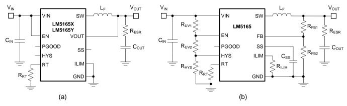
Figure 32. COT Mode Converter Schematics: (a) Fixed Output Voltage of 5 V or 3.3 V, (b) Adjustable Output Voltage With Programmable Soft Start, Current Limit, and UVLO
