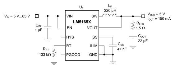
Figure 37. Schematic for Design 1 With  $V_{IN(nom)} = 12 \text{ V}$ ,  $V_{OUT} = 5 \text{ V}$ ,  $I_{OUT(max)} = 150 \text{ mA}$ ,  $F_{SW(nom)} = 220 \text{ kHz}$
