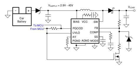
Figure 10-4. Typical Start-Stop Application
