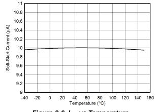
Figure 8-6. I<sub>SS</sub> vs Temperature
