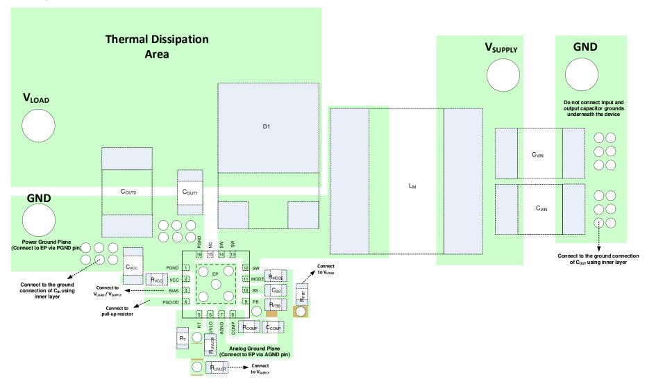
Figure 12-1. PCB Layout Example
