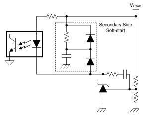
Figure 9-8. Secondary-Side Soft-Start in Flyback
