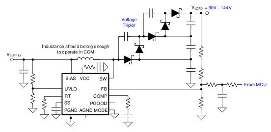
Figure 10-8. LiDAR Bias Supply 2 (CCM Operation)
