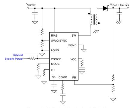
Figure 10-12. Typical Non-Isolated Flyback
