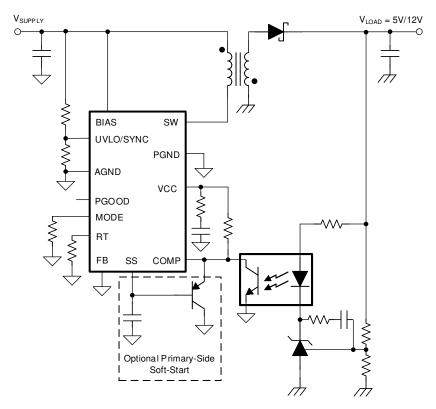
Figure 10-10. Secondary-Side Regulated Isolated Flyback
