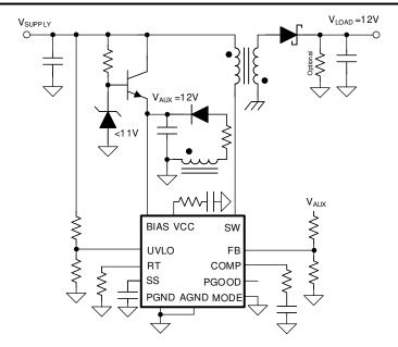
Figure 9-6. External BIAS Supply (PSR Flyback)
