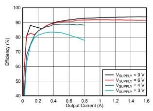
Figure 10-2. Efficiency versus Output Current
