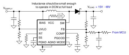
Figure 10-7. LiDAR Bias Supply 1 (DCM Operation)
