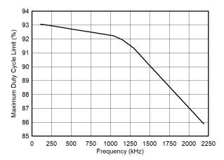
Figure 8-16. Maximum Duty Cycle Limit vs **Frequency**
