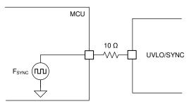
Figure 9-15. Shutdown and Clock Synchronization
