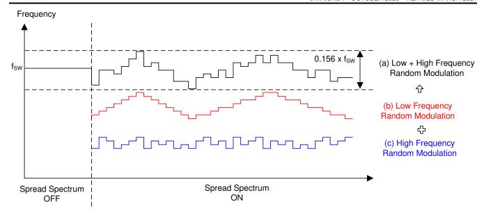
Figure 9-9. Dual Random Spread Spectrum
