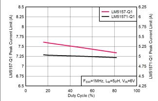
Figure 8-13. Peak Current Limit vs Duty Cycle
