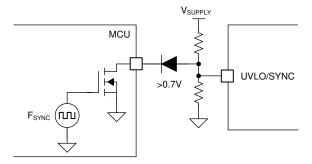
Figure 9-13. UVLO, Standby, and Clock Synchronization (a)
