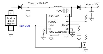
Figure 10-5. Emergency-Call/Boost On-Demand/Portable Speaker
