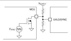
Figure 9-11. UVLO, Shutdown, and Clock Synchronization
