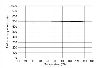
Figure 8-3. BIAS Operating Current vs Temperature
