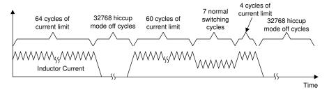
Figure 9-20. Hiccup Mode Overload Protection
