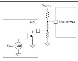
Figure 9-14. UVLO, Standby, and Clock Synchronization (b)
