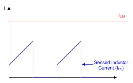
Figure 9-19. Current Sensing (b) at Current Limit Comparator Inputs
