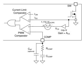
Figure 9-17. Current Sensing and Slope Compensation
