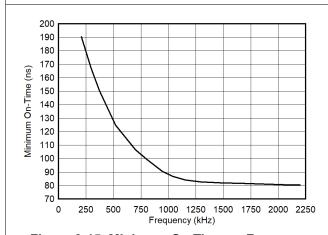
Figure 8-15. Minimum On Time vs Frequency
