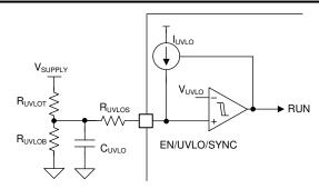
Figure 9-4. Line UVLO using Three UVLO Resistors
