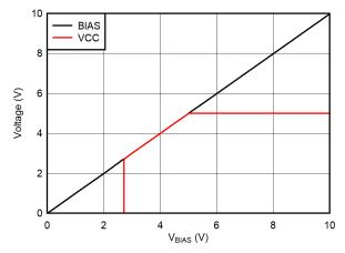
Figure 8-4.  $V_{VCC}$  vs  $V_{BIAS}$
