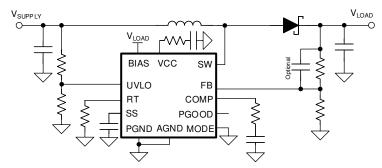
Figure 9-5. Decrease the Minimum Operating Voltage After Start-Up
