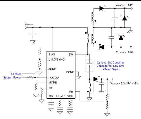
Figure 10-11. Primary-Side Regulated Multiple-Output Isolated Flyback/Isolated SEPIC
