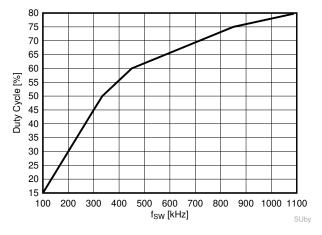
Figure 9-12. Required Duty Cycle to Start-Up by External Synchronization Clock
