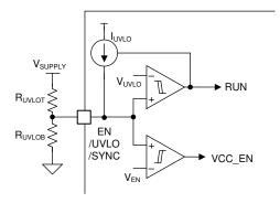
Figure 9-1. Line UVLO and Enable
