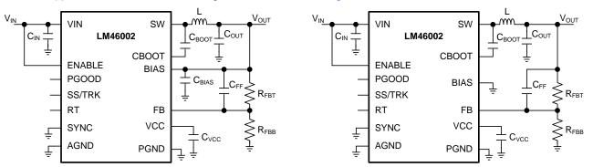
Figure 44. LM46002 Basic Schematic for  $V_{OUT} \ge 3.3 \text{ V}$ , Tie BIAS to  $V_{OUT}$
