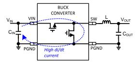
Figure 100. Buck Converter High di / dt Path
