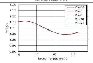
Figure 29. PGOOD Threshold vs Junction Temperature
