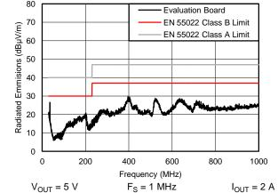
Measured on the LM46002PWPEVM with default BOM. No input filter used.
