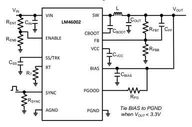
Figure 46. LM46002 Schematic with All Features
