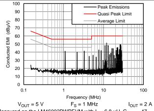
Measured on the LM46002PWPEVM with L = 6.8  $\mu$ H, C<sub>OUT</sub> = 47  $\mu$ F, C<sub>FF</sub> = 47 pF. Input filter L<sub>in</sub> = 1  $\mu$ H C<sub>d</sub> = 47  $\mu$ F C<sub>IN4</sub> = 68  $\mu$ F
