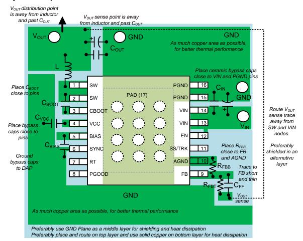
Figure 102. LM46002 PCB Layout Example and Guidelines
