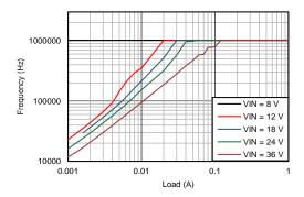
Figure 34. Switching Frequency Decreases with Lower Load Current in PFM Operation  $V_{OUT} = 5 \text{ V}, F_S = 1 \text{ MHz}$
