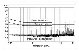
$V_{OUT}$  = 3.3 V  $F_S$  = 500 kHz  $I_{OUT}$  = 1 A Measured on LM46001PWPEVM with default BOM. EVM input filter:  $L_{in}$  = 1  $\mu$ H  $C_d$  = 47  $\mu$ F  $C_{IN4}$  = 68  $\mu$ F
