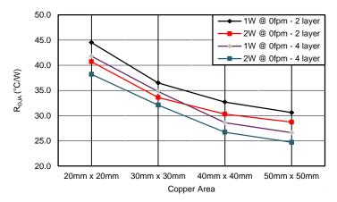
Figure 101. Measured R<sub>0JA</sub> vs PCB Copper Area on a 2-Layer Board and a 4-Layer Board
