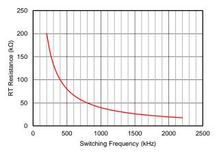
Figure 40. R<sub>T</sub> Resistance vs Switching Frequency
