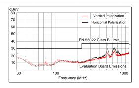
$V_{OUT}$  = 3.3 V  $F_{S}$  = 500 kHz  $I_{OUT}$  = 1 A Measured on the LM46001PWPEVM with default BOM. No input filter used.
