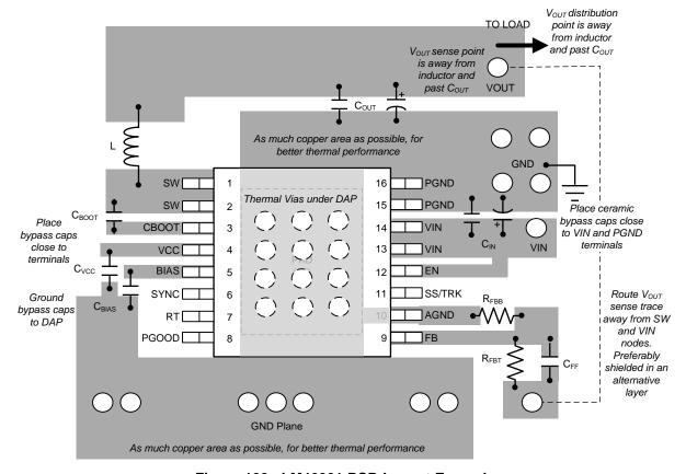
Figure 102. LM46001 PCB Layout Example
