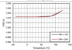
Figure 30. Feedback Voltage vs Junction Temperature
