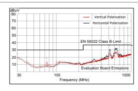
$V_{OUT}=5~V$   $F_S=500~kHz$   $I_{OUT}=1~A$  Measured on the LM46001PWPEVM with L = 27  $\mu H,~C_{OUT}=66~\mu F,~C_{FF}=33~pF.$  No input filter used.
