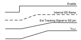
Figure 38. Tracking With Longer Start-up Time Than the Internal Ramp
