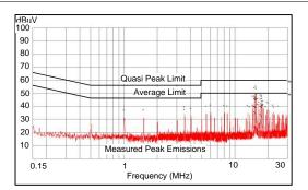
$V_{OUT}=5$  V  $F_S=500$  kHz  $I_{OUT}=1$  Measured on LM46001PWPEVM with L = 27  $\mu H,~C_{OUT}=66~\mu F,~C_{FF}=33~pF.$  EVM input filter L $_{in}=1~\mu H~C_d=47~\mu F~C_{IN4}=68~\mu F$
