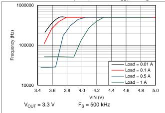
Figure 19. Switching Frequency vs V<sub>IN</sub> in Dropout Operation
