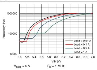
Figure 20. Switching Frequency vs V<sub>IN</sub> in Dropout Operation
