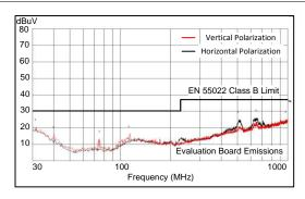
$\rm V_{OUT}=3.3~V~F_{S}=500~kHz~I_{OUT}=0.5~A$  Measured on the LM46000PWPEVM with default BOM. No input filter used.
