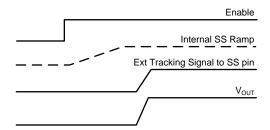
Figure 39. Tracking With Shorter Start-up Time Than the Internal Ramp
