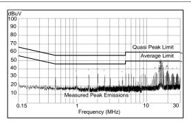
$V_{OUT}$  = 3.3 V  $F_{S}$  = 500 kHz  $I_{OUT}$  = 0.5 A Measured on the LM46000PWPEVM with default BOM. EVM input filter:  $L_{in}$  = 1  $\mu$ H  $C_{d}$  = 47  $\mu$ F  $C_{IN4}$  = 68  $\mu$ F
