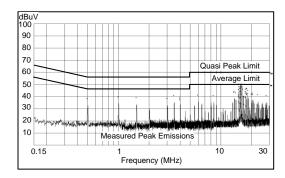
$V_{OUT}=5~V~F_S=500~kHz~I_{OUT}=0.5~A$  Measured on the LM46000PWPEVM with L = 44 µH, C<sub>OUT</sub> = 66 µF, C<sub>FF</sub> = 33 pF. EVM input filter L<sub>in</sub> = 1 µH C<sub>d</sub> = 47 µF C<sub>IN4</sub> = 68 µF.
