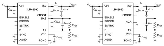
Figure 44. LM46000 Basic Schematic for  $V_{OUT} \ge 3.3 \text{ V}$ , Tie BIAS to  $V_{OUT}$
