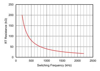
Figure 40. R<sub>T</sub> Resistance vs Switching Frequency
