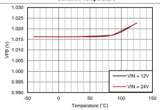
Figure 30. Feedback Voltage vs Junction Temperature
