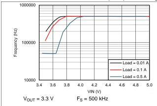
Figure 19. Switching Frequency vs  $V_{\mbox{\scriptsize IN}}$  in Dropout Operation
