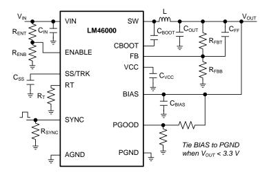
Figure 46. LM46000 Schematic With All Features
