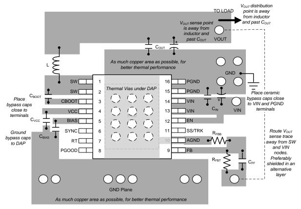
Figure 102. LM46000 PCB Layout Example
