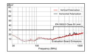
$V_{OUT}$  = 5 V  $F_{S}$  = 500 kHz  $I_{OUT}$  = 0.5 A Measured on the LM46000PWPEVM with L = 44  $\mu\text{H},~C_{OUT}$  = 66  $\mu\text{F},~C_{FF}$  = 33 pF. No input filter used.
