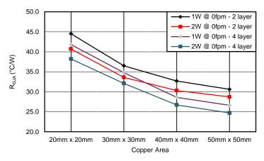
Figure 101. Measured R<sub>0.1A</sub> vs PCB Copper Area on a 2-layer Board and a 4-layer Board
