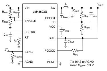
Figure 48. LM43603-Q1 Schematic with All Features
