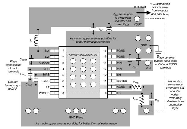
Figure 99. LM43603-Q1 Board Layout Recommendations
