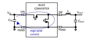
Figure 97. Buck Converter High  $\Delta i/\Delta t$  Path
