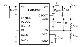
Figure 46. LM43603-Q1 Basic Schematic for  $V_{OUT} \ge 3.3$  V, tie BIAS to  $V_{OUT}$
