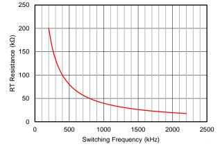
Figure 41. RT vs Frequency Curve
