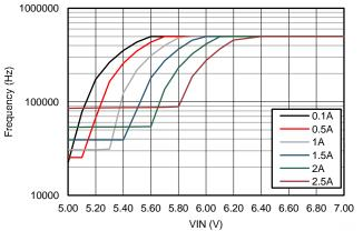
Figure 43.  $V_{OUT} = 5 V Fs = 500 kHz$ Frequency Foldback at Dropout
