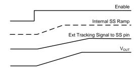
Figure 39. Tracking with Longer Start-up Time than the Internal Ramp
