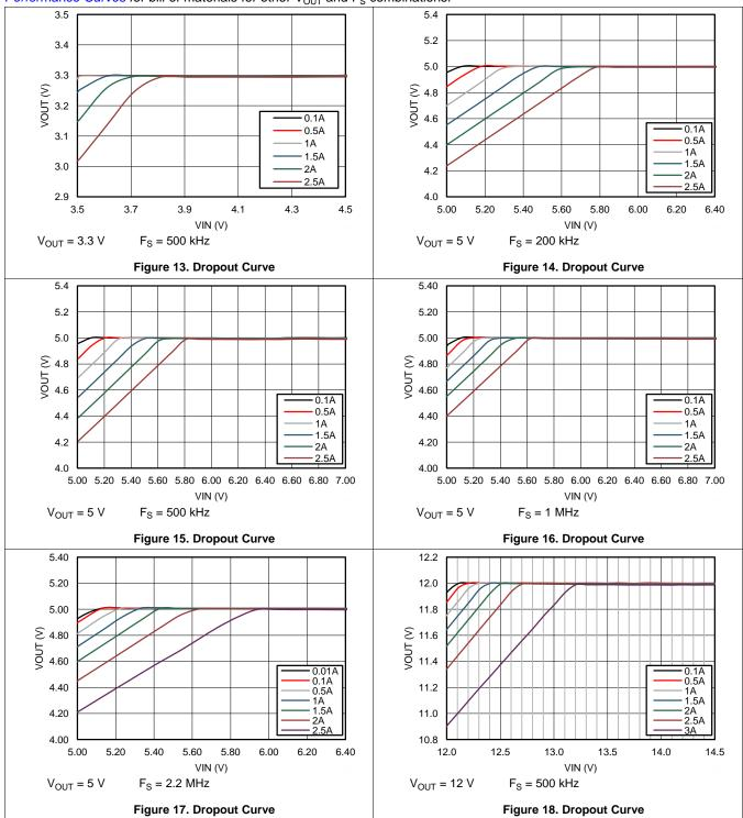
Unless otherwise specified,  $V_{IN} = 12$  V,  $V_{OUT} = 3.3$  V,  $F_S = 500$  kHz, L = 6.8 µH and room temperature. See *Application Performance Curves* for bill of materials for other  $V_{OUT}$  and  $F_S$  combinations.
