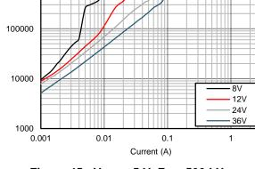
Figure 45.  $V_{OUT} = 5 V$ , Fs = 500 kHz Pulse Frequency Mode Operation
