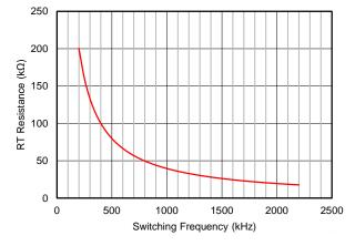
Figure 31. RT vs Frequency Curve
