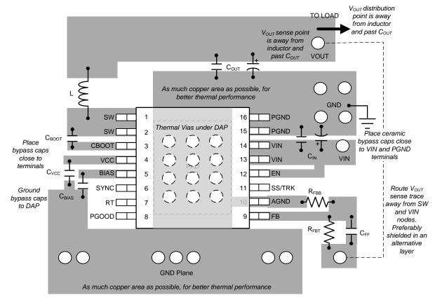
Figure 65. LM43602 Board Layout Recommendations
