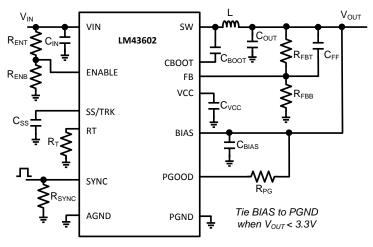
Figure 38. LM43602 Schematic with All Features
