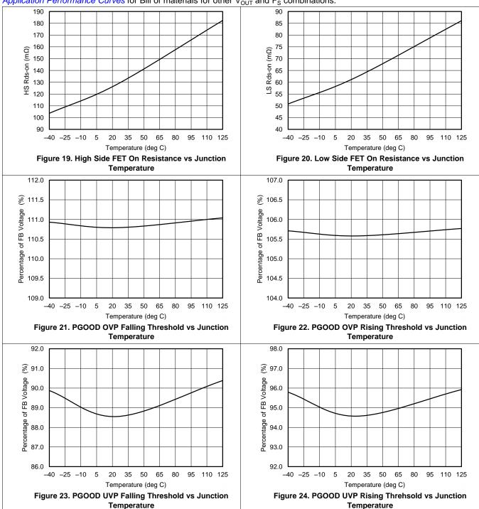
Unless otherwise specified,  $V_{IN} = 12 \text{ V}$ ,  $V_{OUT} = 3.3 \text{ V}$ ,  $F_S = 500 \text{ kHz}$ ,  $L = 6.8 \mu\text{H}$ ,  $C_{OUT} = 120 \mu\text{F}$ ,  $C_{FF} = 100 \text{ pF}$ . See *Application Performance Curves* for Bill of materials for other  $V_{OUT}$  and  $F_S$  combinations.
