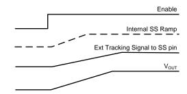
Figure 29. Tracking with Longer Start-up Time Than The Internal Ramp
