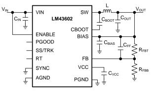
Figure 36. LM43602 Basic Schematic for  $V_{OUT} \ge 3.3$  V, tie BIAS to  $V_{OUT}$
