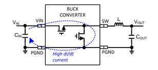
Figure 63. Buck Converter High  $\Delta i/\Delta t$  Path
