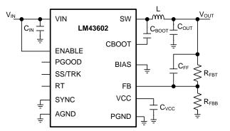
Figure 37. LM43602 Basic Schematic for V<sub>OUT</sub> < 3.3 V, tie BIAS to ground
