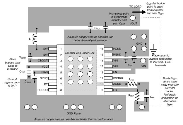
Figure 108. LM43600 PCB Layout Example
