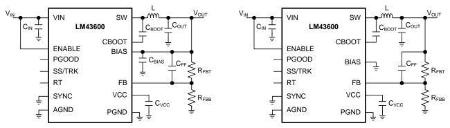
Figure 44. LM43600 Basic Schematic for V<sub>OUT</sub> ≥ 3.3 V, Tie BIAS to V<sub>OUT</sub>
