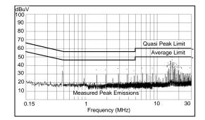
$V_{OUT}$  = 3.3 V  $F_{SW}$  = 500 kHz  $I_{OUT}$  = 0.5 A Measured on the LM43600PWPEVM with default BOM. Input filter:  $L_{in}$  = 1  $\mu$ H  $C_d$  = 47  $\mu$ F  $C_{IN4}$  = 68  $\mu$ F
