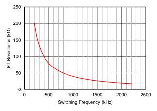
Figure 40. R<sub>T</sub> Resistance vs Switching Frequency
