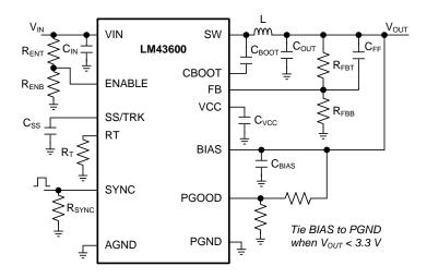
Figure 46. LM43600 Schematic with All Features
