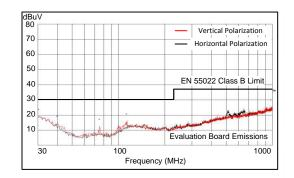
$V_{OUT}$  = 3.3 V  $F_{SW}$  = 500 kHz  $I_{OUT}$  = 0.5 A Measured on the LM43600PWPEVM with default BOM. No input filter used
