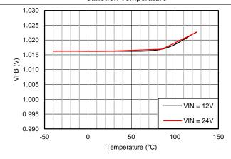
Figure 30. Feedback Voltage vs Junction Temperature
