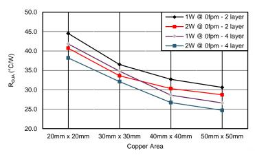
Figure 107. Measured R<sub>0.1A</sub> vs PCB Copper Area on a 2-layer Board and a 4-layer Board
