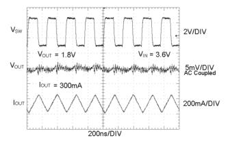
Figure 42. Typical PWM Operation
