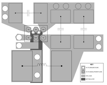
Figure 53. LM3291 Layout Example
