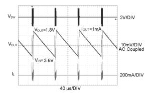
Figure 43. Typical ECO Operation
