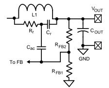
Figure 15. Type III Ripple Circuit
