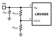
Figure 10. UVLO Resistor Setting
