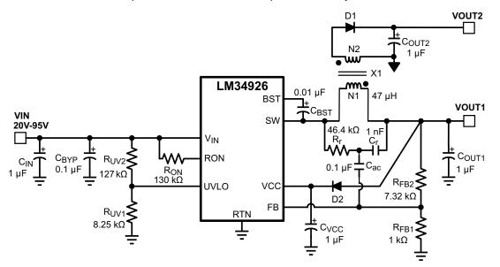
Figure 12. Isolated Fly-Buck™ Converter Using LM34926
