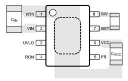
Figure 18. Placement of Bypass Capacitors
