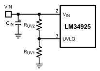
Figure 10. UVLO Resistor Setting
