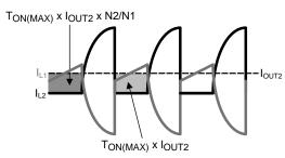
Figure 13. Current Waveforms for C<sub>OUT1</sub> Ripple Calculation
