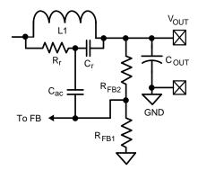
Figure 15. Type III Ripple Circuit
