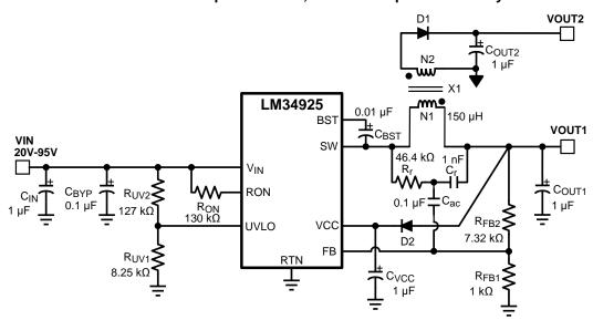
Figure 12. Isolated Fly-Buck Converter Using LM34925
