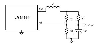
Figure 13. Alternate Minimum Output Ripple
