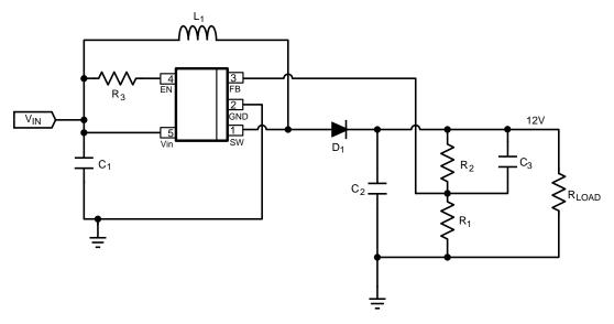
Figure 23. LM2735Y (520 kHz):  $V_{IN}$  = 5 V,  $V_{OUT}$  = 12 V at 350 mA
