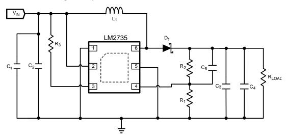
Figure 32. LM2735Y (520 kHz):  $V_{IN}$  = 3.3 V,  $V_{OUT}$  = 20 V at 150 mA
