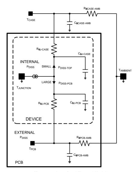
Figure 48. Associated Thermal Model
