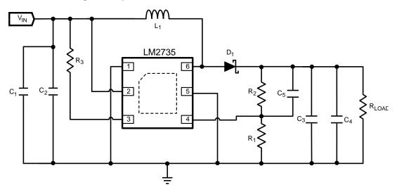
Figure 25. LM2735Y (520 kHz):  $V_{IN}$  = 3.3 V,  $V_{OUT}$  = 12 V at 350 mA
