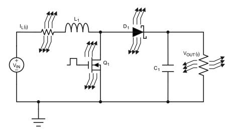
Figure 47. Thermal Schematic
