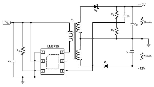
Figure 36. LM2735Y (520 kHz):  $V_{IN} = 5 \text{ V}$ ,  $V_{OUT} = \pm 12 \text{ V}$  150 mA
