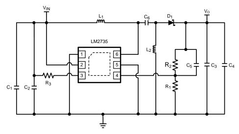
Figure 39. SEPIC Converter Schematic
