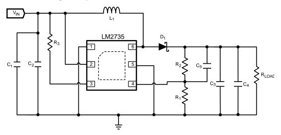
Figure 24. LM2735X (1.6 MHz):  $V_{IN}$  = 3.3 V,  $V_{OUT}$  = 12 V at 350 mA
