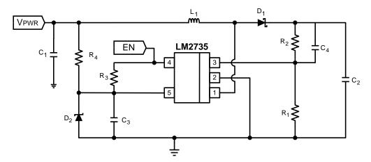
Figure 37. LM2735X (1.6 MHz):  $V_{PWR} = 9 V$ ,  $V_{OUT} = 12 V$  at 500 mA
