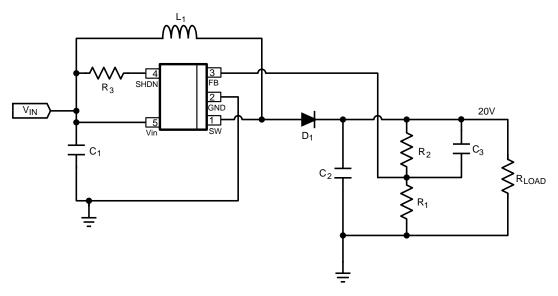
Figure 29. LM2735X (1.6 MHz):  $V_{IN}$  = 3.3 V,  $V_{out}$  = 20 V at 100 mA
