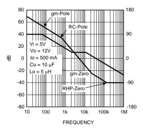
Figure 15. LM2735 Without External Compensation
