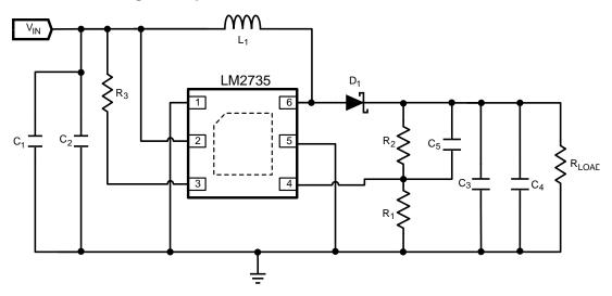
Figure 31. LM2735X (1.6 MHz):  $V_{IN}$  = 3.3 V,  $V_{OUT}$  = 20 V at 150 mA
