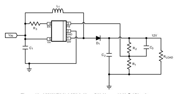
Figure 18. LM2735X (1.6 MHz):  $V_{IN} = 5 \text{ V}$ ,  $V_{OUT} = 12 \text{ V}$  @ 350 mA
