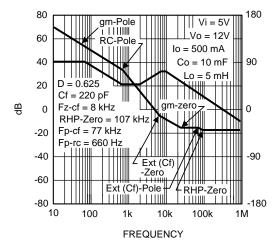
Figure 16. LM2735 With External Compensation
