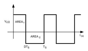
Figure 40. Inductor Volt-Sec Balance Waveform
