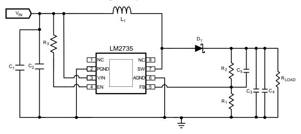
Figure 26. LM2735Y (520 kHz):  $V_{IN}$  = 3.3 V,  $V_{OUT}$  = 12 V at 350 mA
