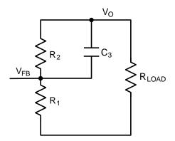
Figure 17. Setting External Pole-Zero
