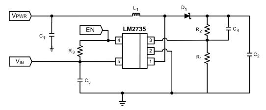
Figure 38. LM2735X (1.6 MHz):  $V_{PWR} = 9 \text{ V in} = 2.7 \text{ V} - 5.5 \text{ V}$ ,  $V_{OUT} = 12 \text{ V at } 500 \text{ mA}$
