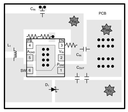
Figure 44. Example of Proper PCB Layout
