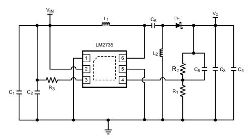
Figure 33. LM2735X (1.6 MHz):  $V_{IN}$  = 2.7 V - 5 V,  $V_{OUT}$  = 3.3 V at 500 mA
