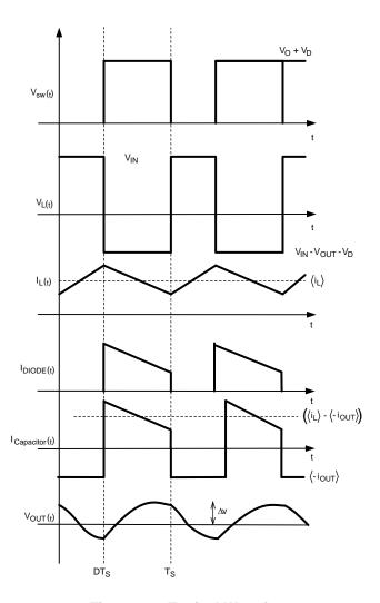
Figure 14. Typical Waveforms
