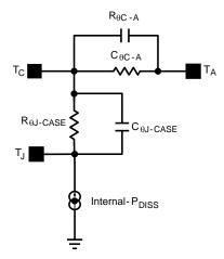
Figure 46. Simplified Thermal Impedance Model
