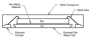
Figure 42. Internal WSON Connection
