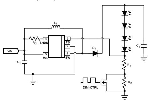
Figure 35. LM2735X (1.6 MHz):  $V_{IN}$  = 2.7 V - 5 V,  $V_{OUT}$  = 20 V at 50 mA
