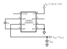
Figure 28. Splitting V<sub>IN</sub> in Half
