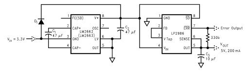
Figure 23. Generating +5 V From +3.3 V Input Voltage
