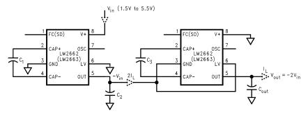
Figure 19. Increasing Output Voltage by Cascading Devices
