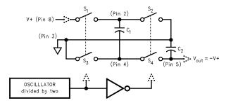
Figure 16. Voltage Inverting Principle
