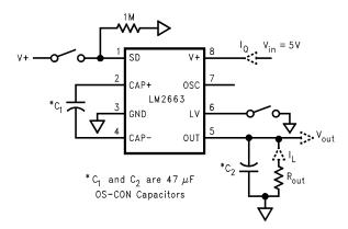
Figure 15. LM2663 Test Circuit
