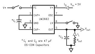
Figure 14. LM2662 Test Circuit
