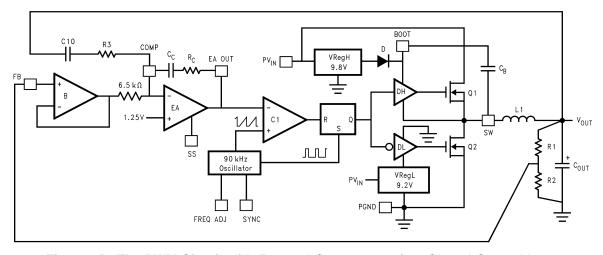
Figure 15. The PWM Circuit with External Components in a Closed Control Loop
