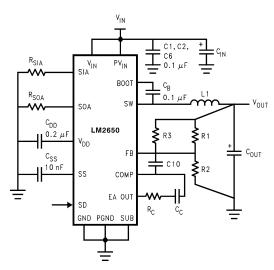
Figure 18. The Typical 90 kHz Application Circuit
