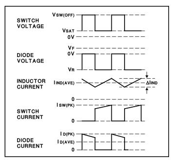
Figure 2. Step-up Regulator Waveforms
