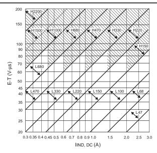
Note: This chart assumes that the inductor ripple current inductor is approximately 20% to 30% of the average inductor current (when the regulator is under full load). Greater ripple current causes higher peak switch currents and greater output ripple voltage. Lower ripple current is achieved with larger value inductors. The factor of 20% to 30% is chosen as a convenient balance between the two extremes.
