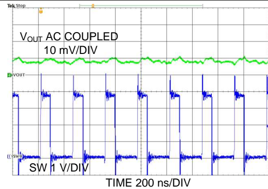
Figure 41. Output Voltage Ripple, PWM Mode. I_{OUT} = 200 mA ; One Phase Active
