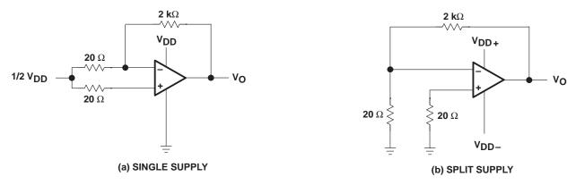
Figure 36. Noise-Test Circuit
