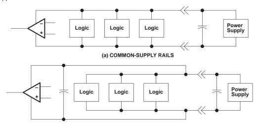
(b) SEPARATE-BYPASSED SUPPLY RAILS (preferred)
