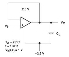
Figure 45. Test Circuit for Output Characteristics
