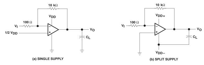
Figure 37. Gain-of-100 Inverting Amplifier
