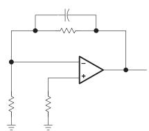
Figure 43. Compensation for Input Capacitance
