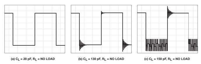
Figure 46. Effect of Capacitive Loads
