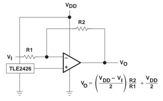
Figure 40. Inverting Amplifier With Voltage Reference
