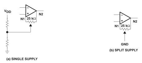
Figure 99. Input Offset Voltage Null Circuit
