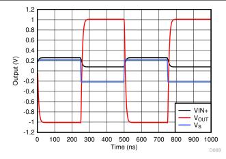
Figure 8-8. I/O Swing Simulation Using the TINA-TI™ Model
