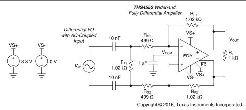
Figure 8-10. Example AC-Coupled Differential Input Design
