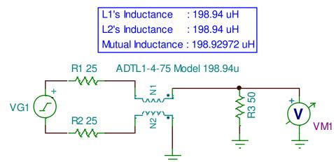
Figure 7-2. Output Measurement Balun Simulation Circuit in TINA-TI™
