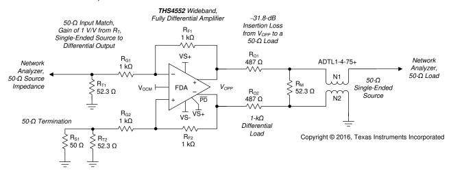
Figure 7-1. Single-Ended Source to a Differential Gain of a 1 V/V Test Circuit
