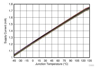
Figure 10-1. Linear Temperature Coefficient for Supply Current
