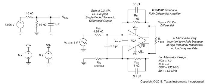
Figure 8-6. DC-Coupled, Single-Ended to Differential Attenuator Design
