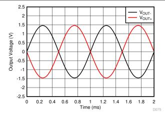
Figure 9-19. Output Waveform of the DAC Output Driver
