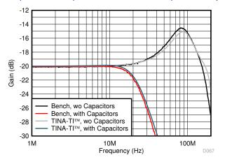
Figure 9-9. Attenuator Response Shapes With and Without External Capacitors
