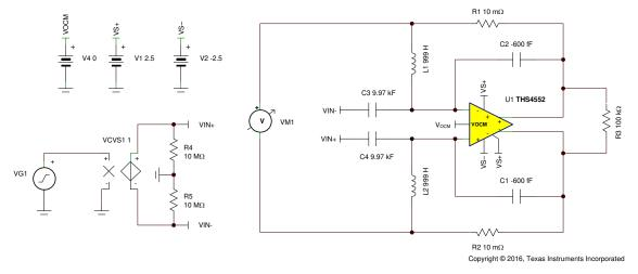
Figure 12-1. Open-Loop Gain and Phase TINA-TI™ Simulation Setup
