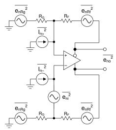
Figure 9-1. FDA Noise Analysis Circuit
