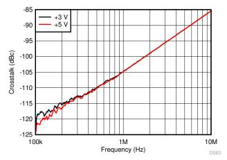
Figure 9-4. THS4552PW Crosstalk vs Frequency
