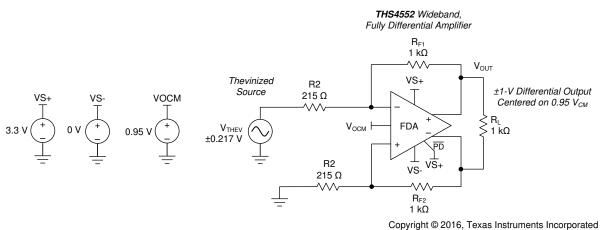
Figure 8-7. Input V<sub>ICM</sub> Analysis Circuit From the Design of Figure 9-20
