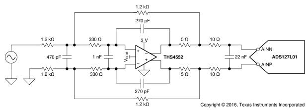
Figure 9-2. 500-kHz Low-Pass Active Filter
