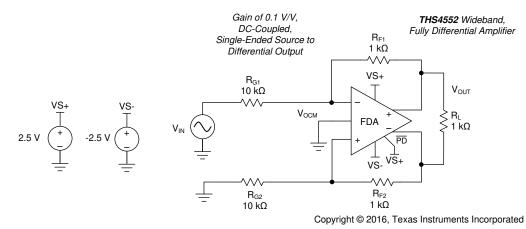
Figure 9-7. Divide-by-10 Attenuator Application for the THS4552
