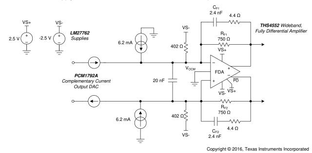
Figure 9-17. PCM1792A DAC Output Driver
