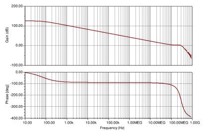
Figure 12-2. Open-Loop Gain and Phase Simulation Result
