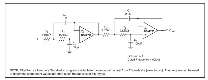
Figure 7. Four-Pole Butterworth Sallen-Key Low-Pass Filter
