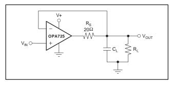
Figure 3. Series Resistor in Unity-Gain Buffer Configuration Improves Capacitive Load Drive
