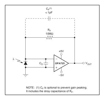
Figure 5. Dual-Supply Transimpedance Amplifier
