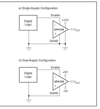
Figure 1. Enable Reference Pin Connection for Single- and Dual-Supply Configurations
