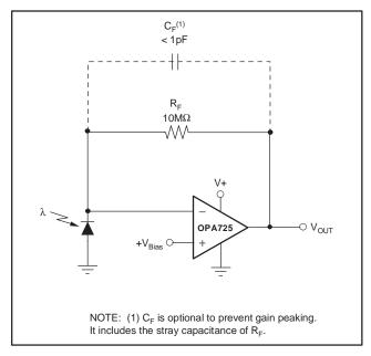
Figure 6. Single-Supply Transimpedance Amplifier
