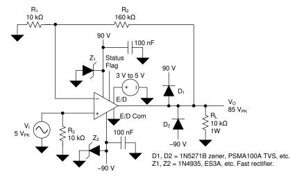
Figure 61. OPA462, High-Voltage Noninverting Amplifier,  $A_V = 17 V/V$
