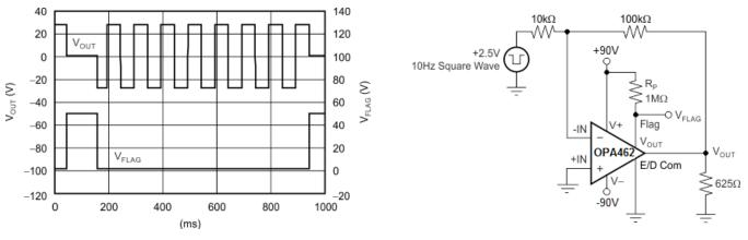
Figure 68. Thermal Shutdown
