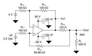
Figure 63. High-Voltage, 20-mA, Improved Howland Current Pump
