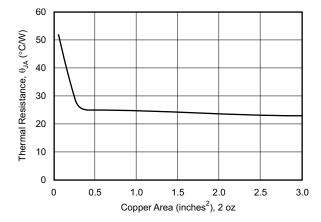
Figure 69. Thermal Resistance vs Circuit Board Copper Area
