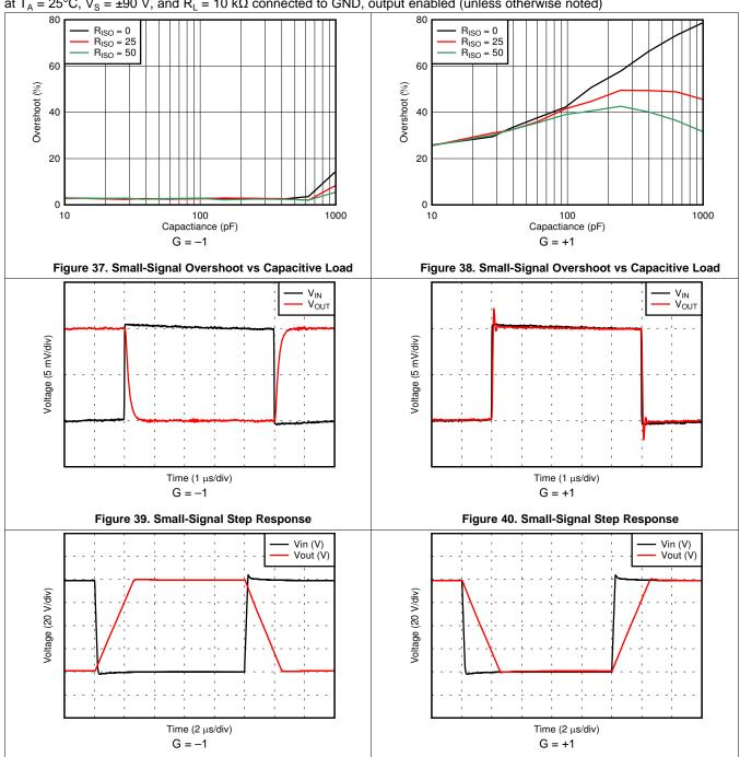
at  $T_A = 25^{\circ}$ C,  $V_S = \pm 90$  V, and  $R_L = 10 \text{ k}\Omega$  connected to GND, output enabled (unless otherwise noted)
