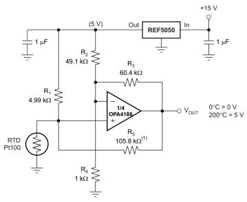
(1) R<sub>5</sub> provides positive-varying excitation to linearize output.
