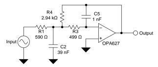
Figure 44. 25-kHz Low Pass Filter
