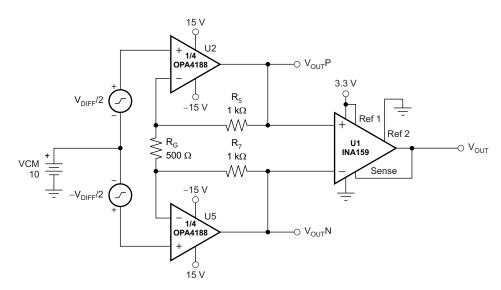
Figure 46. Discrete INA + Attenuation for ADC With a 3.3-V Supply Circuit
