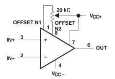
Figure 2. Input Offset-Voltage Null Circuit
