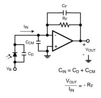
Figure 1. Photodiode Transimpedance Amplifier
