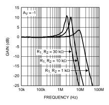
Figure 47. Gain Peaking Caused by Large R<sub>1</sub>, R<sub>2</sub>
