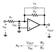
Figure 46. Inverting Amplifier
