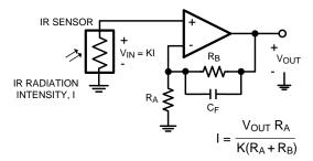
Figure 59. IR Radiation Sensor
