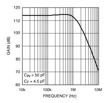
Figure 58. 1.5 MHz Transimpedance Amplifier Frequency Response
