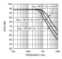
Figure 56. Frequency Response for  $A_{TI} = 47000$
