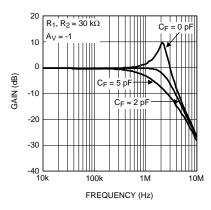
Figure 48. Gain Peaking Eliminated by C<sub>F</sub>
