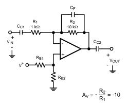
Figure 49. Inverting Audio Preamplifier
