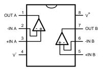
Figure 4. 8-Pin VSSOP Top View
