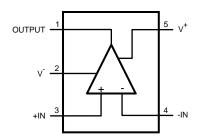
Figure 3. 5-Pin SOT-23 Top View
