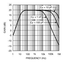
Figure 51. Frequency Response of the Inverting Audio Preamplifier
