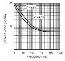
Figure 2. Input Referred Voltage Noise vs. Frequency
