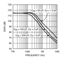
Figure 55. Frequency Response for  $A_{TI} = 470000$
