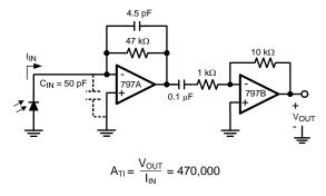
Figure 57. 1.5 MHz Transimpedance Amplifier with  $A_{TI} = 470000$
