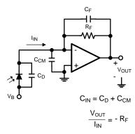
Figure 52. Photodiode Transimpedance Amplifier
