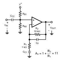
Figure 50. Non-inverting Audio Preamplifier
