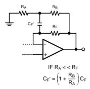
Figure 54. Obtaining Small C<sub>F</sub> from Large C<sub>F</sub>'
