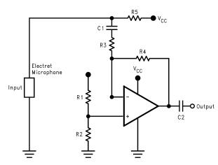
Figure 1. A Battery Powered Microphone Preamplifier
