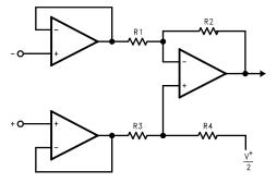
Figure 28. Three-op-amp Instrumentation Amplifier
