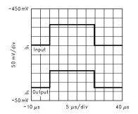
Figure 24. Pulse Response of the LMV721-N Circuit in Figure 23
