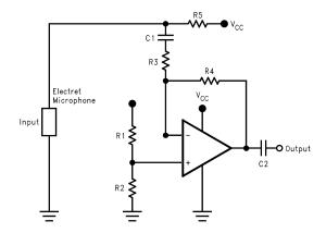
Figure 33. A Battery Powered Microphone Preamplifier
