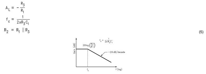
Figure 32. Frequency Response of Simple Low-pass Active Filter in Figure 31
