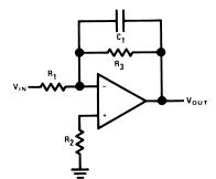
Figure 31. Simple Low-Pass Active Filter
