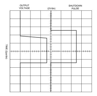
Figure 31. Output Recovery from Shutdown
