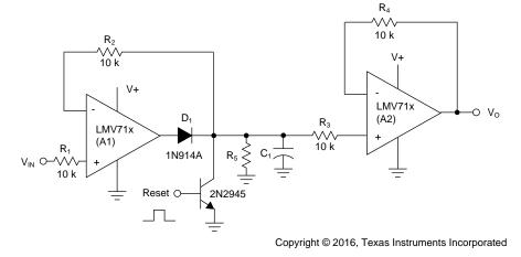
Figure 36. Peak Detector Schematic
