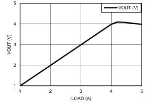
Figure 35. High-Side Current-Sensing Results
