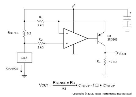
Figure 34. High-Side, Current-Sensing Schematic
