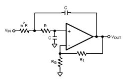
Figure 40. Sallen-Key Low-Pass Filter
