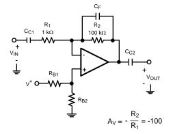
Figure 37. High Gain Inverting Amplifier
