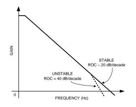
Figure 34. Gain vs Frequency for an Operational Amplifiers
