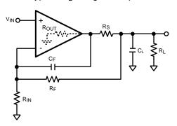
Figure 35. In-the-Loop Compensation
