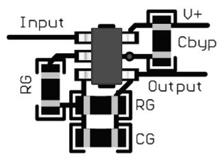
Figure 41. LMV65x Layout Example
