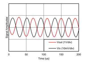
Figure 38. High Gain Inverting Amplifier Results
