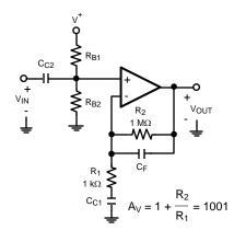
Figure 39. High Gain Noninverting Amplifier
