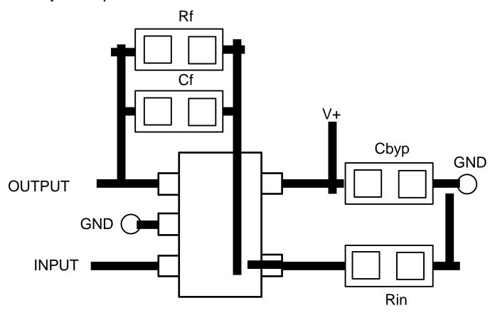
Figure 47. LMV641 Layout Example
