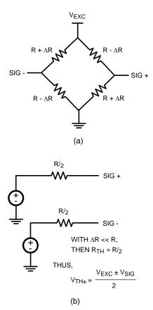
Figure 42. Anisotropic Magnetoresistive Wheatstone Bridge Sensor, (a), and Thevenin Equivalent Circuit, (b)
