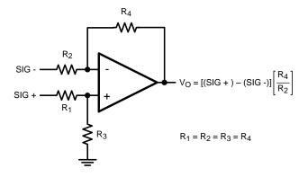
Figure 43. Differential Input Amplifier
