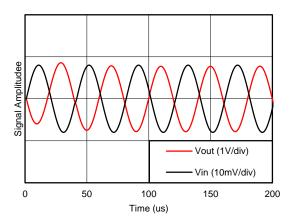
Figure 40. High Gain Inverting Amplifier Results
