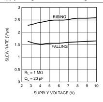
Figure 35. Slew Rate vs Supply Voltage
