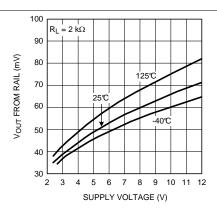
Figure 31. Output Swing High vs Supply Voltage
