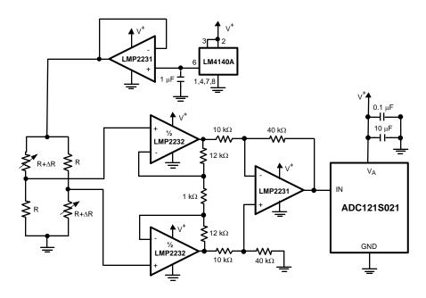
Figure 1. Strain Gauge Bridge Amplifier
