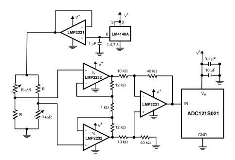
Figure 52. Strain Gauge Bridge Amplifier
