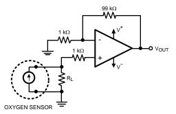
Figure 53. Precision Oxygen Sensor
