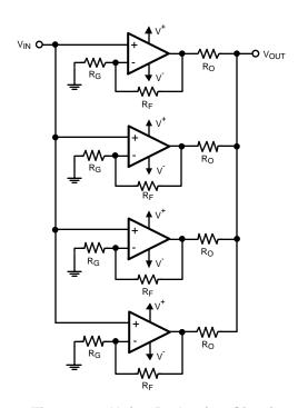
Figure 49. Noise Reduction Circuit
