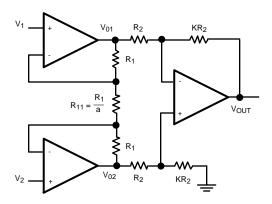
Figure 50. Instrumentation Amplifier
