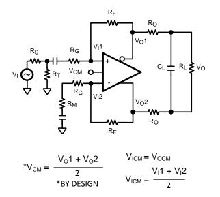
Figure 30. AC-Coupled for Single Supply Operation
