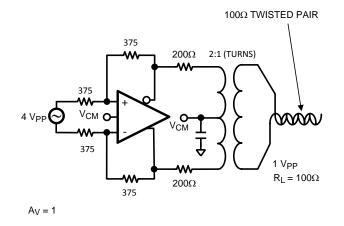
Figure 34. Transformer Out Low-Impedance Load
