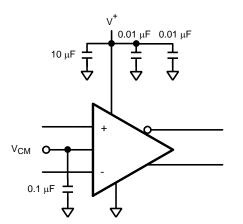
Figure 26. Single Supply Bypassing Capacitors
