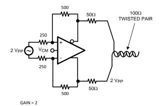
Figure 24. Fully Differential Cable Driver
