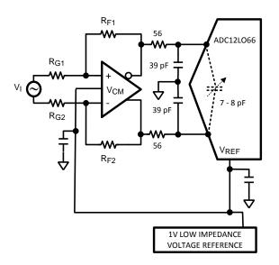
Figure 31. Driving an ADC
