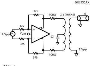
GAIN = 1C<sub>1</sub> IS NOT REQUIRED IF V<sub>CM</sub> = GROUND
