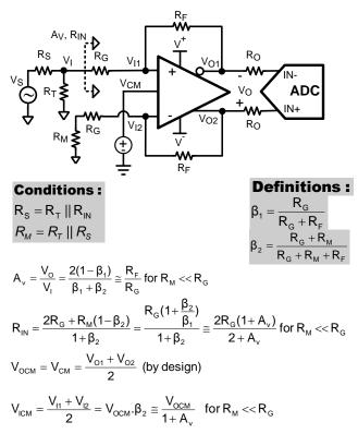
Figure 28. Single-Ended Input to Differential Output Schematic
