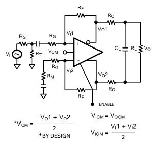
Figure 29. AC-Coupled for Single Supply Operation
