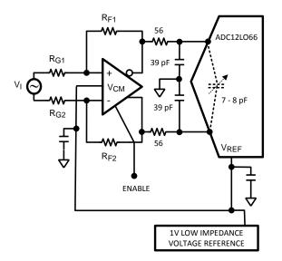
Figure 27. Driving an ADC
