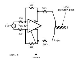
Figure 22. Fully Differential Cable Driver
