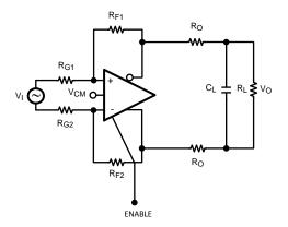
Figure 21. Typical Fully Differential Application Schematic
