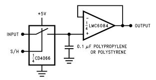
Figure 32. Low-Leakage Sample and Hold
