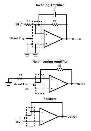
Figure 29. Typical Connections of Guard Rings
