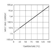
Figure 2. Input Bias Current vs Temperature
