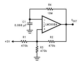
Figure 33. 1 Hz Square Wave Oscillator
