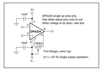
FIGURE 1. OPA234 Offset Voltage Trim Circuit.
