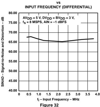
SIGNAL-TO-NOISE AND DISTORTION
