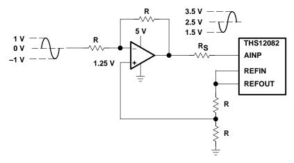
Figure 17. Level-Shift for DC-Coupled Input
