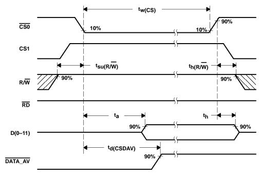
Figure 11. Read Timing Diagram Using R/W (CSO-controlled)
