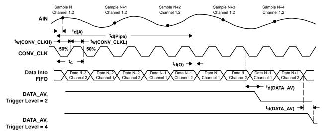
Figure 3. Timing of Continuous Conversion Mode (2-channel operation)
