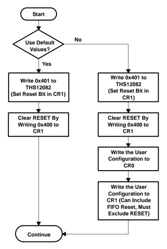
Figure 9. THS12082 Configuration Flow
