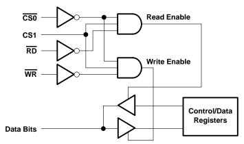
Figure 10. Logical Combination of CSO, CS1, RD, and WR
