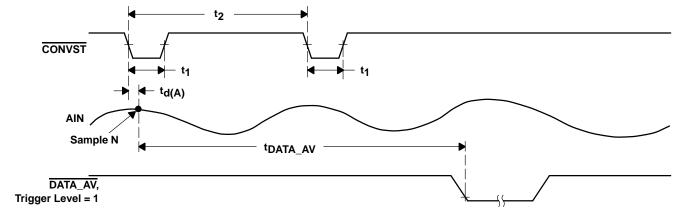
Figure 1. Timing of Single Conversion Mode
