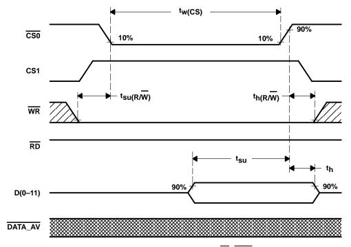
Figure 12. Write Timing Diagram Using R/W (CS0-controlled)
