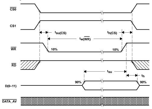
Figure 14. Write Timing Diagram Using WR (WR-controlled)
