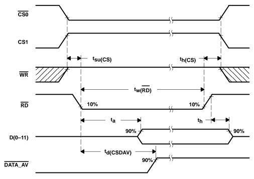
Figure 13. Read Timing Diagram Using RD (RD-controlled)
