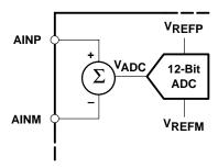
Figure 16. Differential Input Stage
