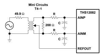
Figure 18. Transformer Coupled Input
