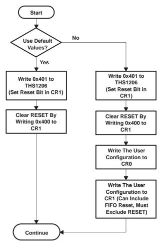
Figure 11. THS1206 Configuration Flow
