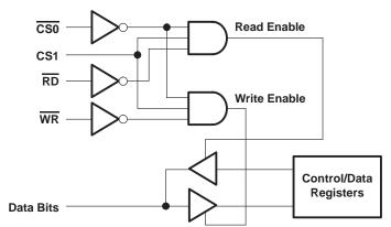
Figure 12. Logical Combination of CS0, CS1, RD, and WR
