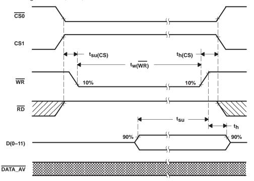
Figure 16. Write Timing Diagram Using WR (WR-controlled)
