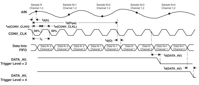
Figure 3. Timing of Continuous Conversion Mode (2-channel operation)
