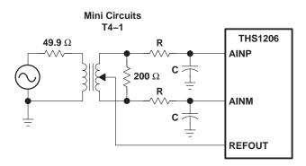
Figure 20. Transformer Coupled Input
