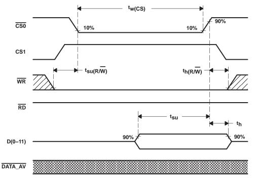
Figure 14. Write Timing Diagram Using R/W (CS0-controlled)
