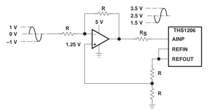
Figure 19. Level-Shift for DC-Coupled Input
