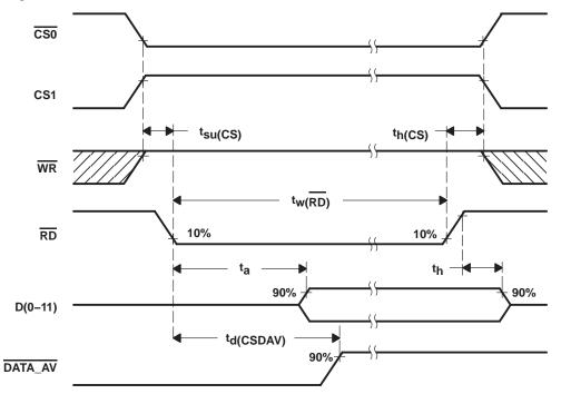
Figure 15. Read Timing Diagram Using RD (RD-controlled)
