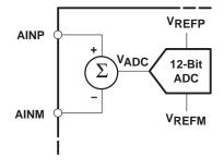
Figure 18. Differential Input Stage
