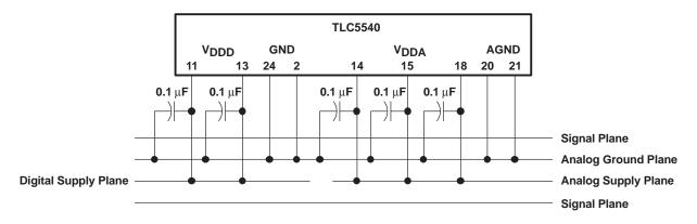
Figure 11. AV<sub>DD</sub>, DV<sub>DD</sub>, AGND, and DGND Connections
