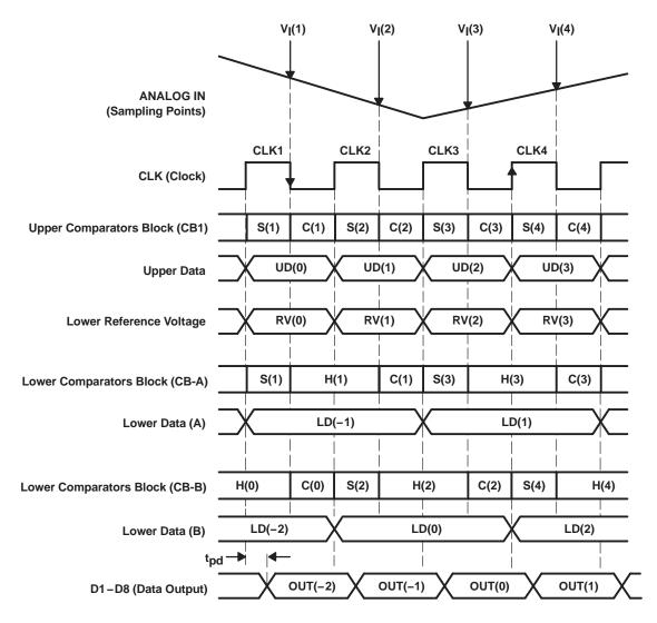
Figure 12. Internal Functional Timing Diagram
