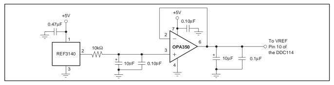
Figure 6. Recommended External Voltage Reference Circuit for Best Low-Noise Operation with the DDC114
