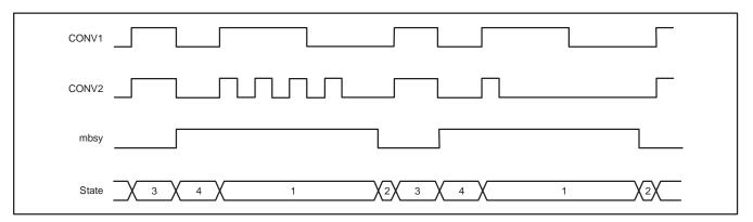
Figure 16. Equivalent CONV Signals in Non-Continuous Mode
