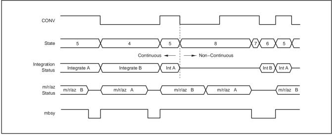
Figure 18. Changing from Continuous Mode to Non-Continuous Mode
