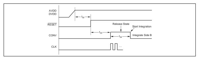
Figure 28. Timing Diagram at Power-Up of the DDC114
