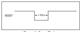
Figure 9. Reset Timing
