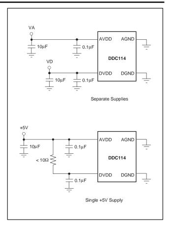
Figure 27. Power-Supply Connection Options
