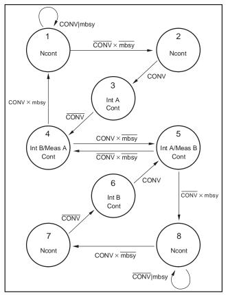
Figure 10. Integrate/Measure State Diagram
