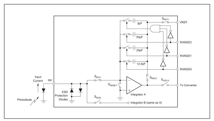
Figure 3. Basic Integration Configuration for Input 1, Shown with a 250pC (C<sub>F</sub> = 62.5pF) Input Range
