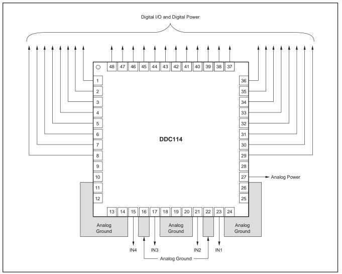
Figure 29. Recommended Shield for DDC114 Layout Design
