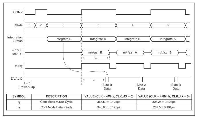
Figure 11. Continuous Mode Timing
