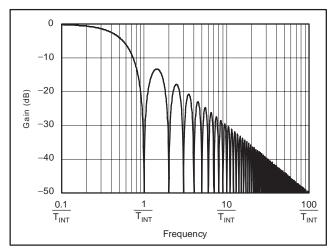
Figure 7. Frequency Response of the DDC114
