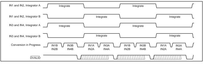
Figure 2. Basic Integration and Conversion Timing for the DDC114 (continuous mode)
