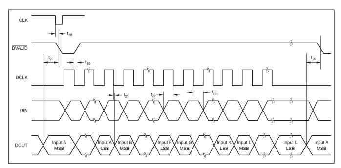
Figure 22. Timing Diagram When Using the DIN Function of the DDC114
