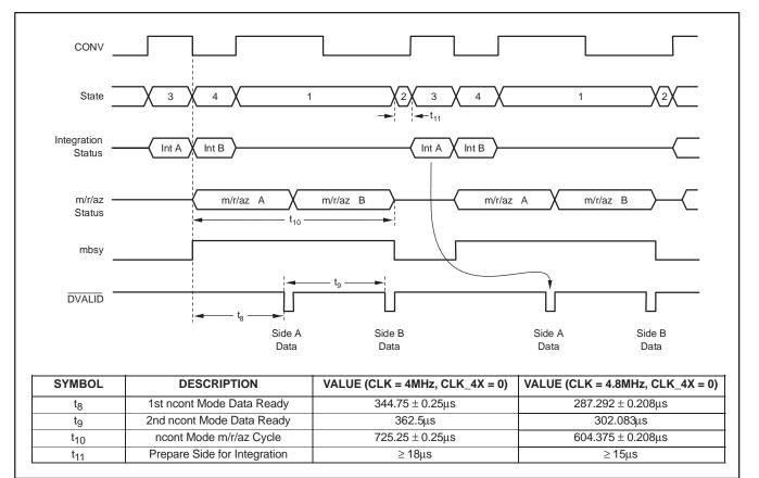
Figure 13. Non-Continuous Mode Timing
