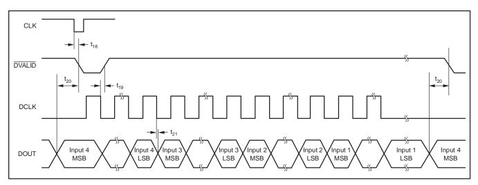
Figure 20. Digital Interface Timing Diagram for Data Retrieval From a Single DDC114
