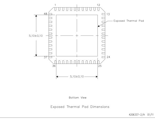
NOTE: All linear dimensions are in millimeters
