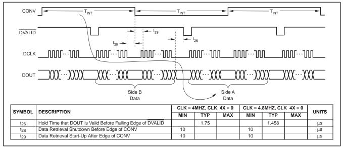
Figure 25. Readback Before and After CONV Toggles
