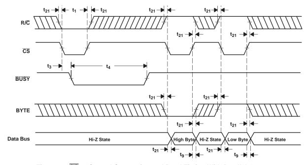
Figure 31. CS to Control Conversion and Read Timing With Parallel Outputs
