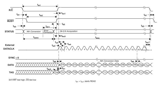
Figure 35. Read After Conversion (Discontinuous External DATACLK)
