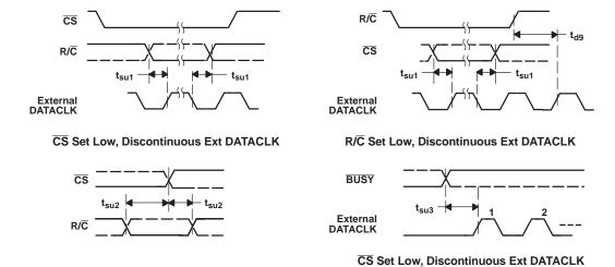
**Figure 32. Critical Timing Parameters**
