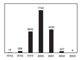
Figure 43. Histogram of 16,384 Conversions with V<sub>IN</sub> = 0 V in ±10 V Bipolar Range
