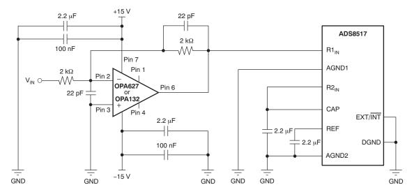
Figure 40. Typical Driving Circuit (±10 V, No Trim)
