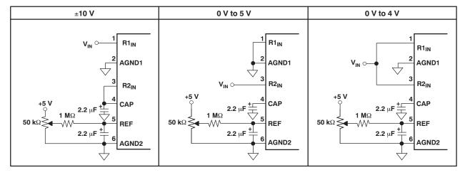
Figure 38. Circuit Diagrams (with Gain Adjust Trim)
