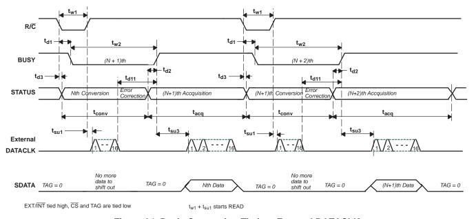
Figure 34. Basic Conversion Timing: External DATACLK
