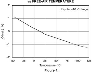
BIPOLAR POSITIVE FULL-SCALE ERROR VS FREE-AIR TEMPERATURE
