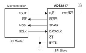
NOTE: CPOL = 0 (inactive SCLK is LOW) CPHA = 1 (data valid on SCLK falling edge)
