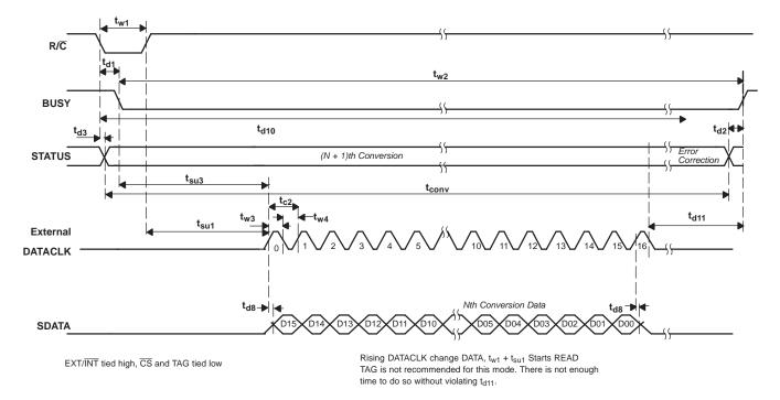
Figure 36. Read During Conversion (Discontinuous External DATACLK)
