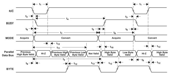
Figure 30. Conversion Timing With Parallel Output (CS and DATACLK Tied Low, EXT/INT Tied High)
