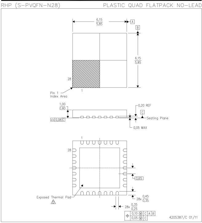
NOTES: All linear dimensions are in millimeters. Dimensioning and tolerancing per ASME Y14.5M—1994. This drawing is subject to change without notice. QFN (Quad Flatpack No—Lead) Package configuration.
