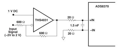
Figure 52. Bipolar Input Drive Configuration
