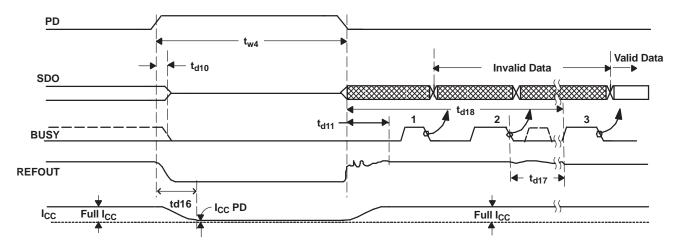
Figure 53. Device Full Power Down/Resume (Internal Refernce Used)
