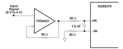
Figure 51. Unipolar Input Drive Configuration
