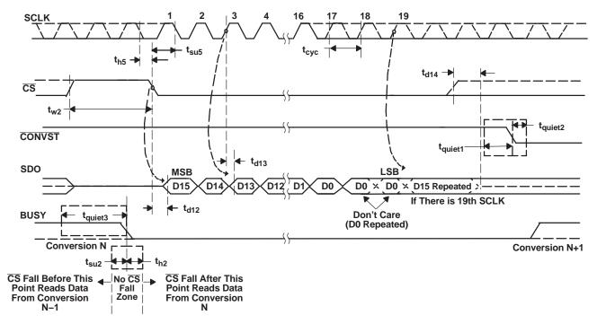
Figure 45. Read Frame Controlled via  $\overline{CS}$  (FS = 1)
