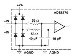
Figure 50. Simplified Analog Input
