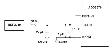
Figure 49. ADS8370 Using External Reference
