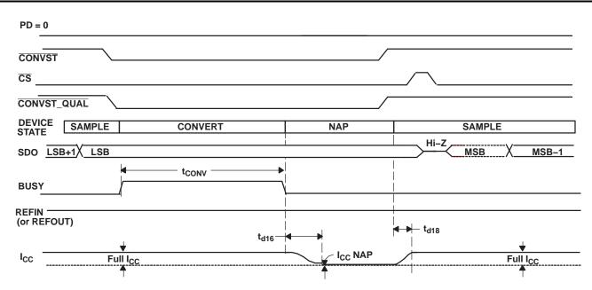
Figure 55. Device Nap Power Down/Resume
