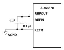
Figure 48. ADS8370 Using Internal Reference
