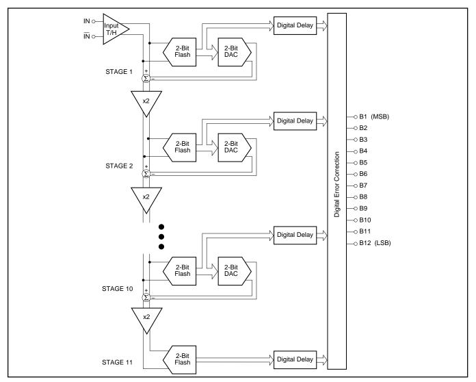
FIGURE 2. Pipeline A/D Converter Architecture.
