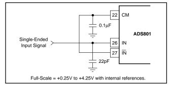
FIGURE 7. Single-Ended Input Connection.
