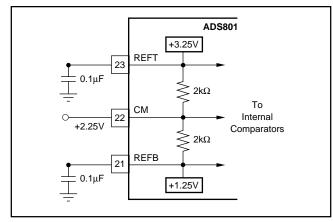
FIGURE 3. Internal Reference Structure.
