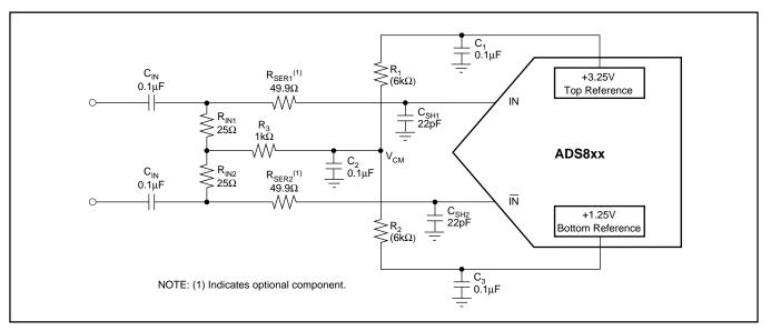
FIGURE 5. AC-Coupled Differential Input Circuit.
