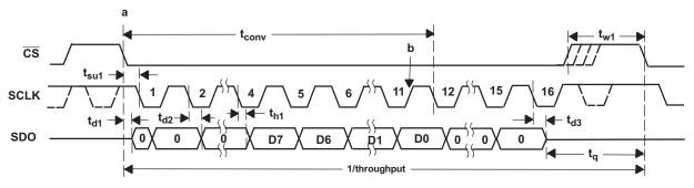
Figure 33. ADS7888 Interface Timing Diagram
