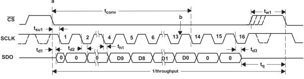
Figure 32. ADS7887 Interface Timing Diagram
