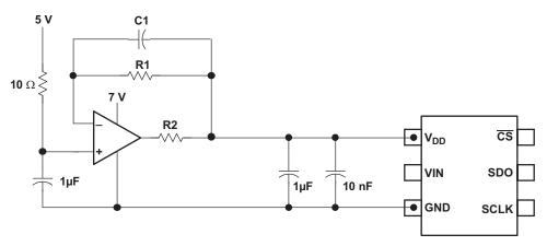
Figure 42. Buffering With the OPA735
