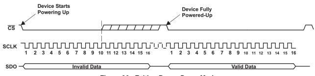
Figure 36. Exiting Power-Down Mode
