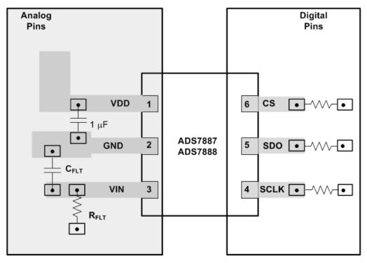
Figure 43. ADS7887 and ADS7888 Example Layout
