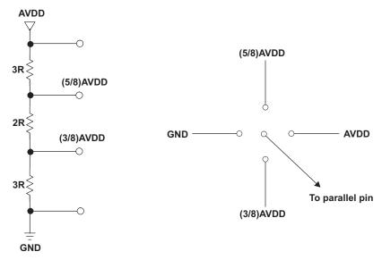
Figure 7. Simple Scheme to Configure 4-Level Control Pins
