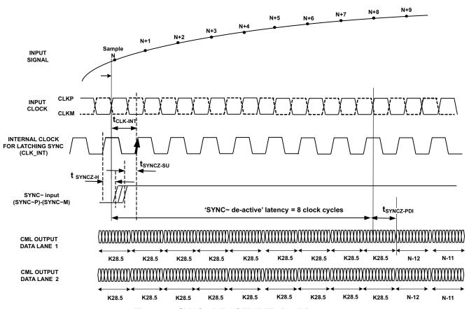
Figure 6. SYNC~ DE-ACTIVE Timing Diagram
