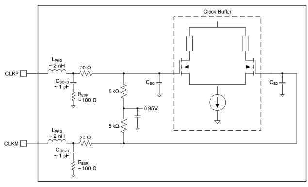
Note: C<sub>EQ</sub> is 1pF to 3pF and is the equivalent input capacitance of the clock buffer.
