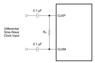
Figure 49. Differential Sine-Wave Clock Driving Circuit
