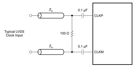
Figure 50. LVDS Clock Driving Circuit
