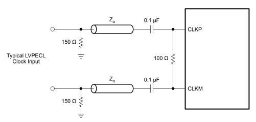
Figure 51. LVPECL Clock Driving Circuit
