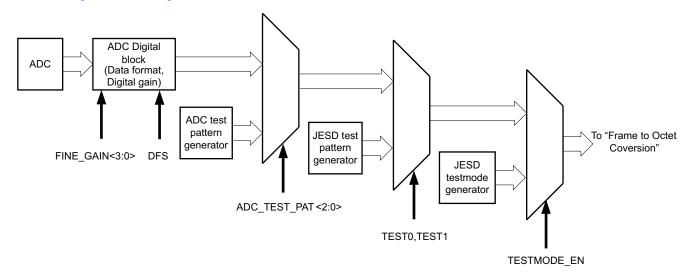
Figure 10. Register Modes Preceding Frame to Octet Conversion Block
