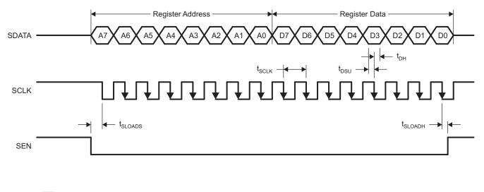
Figure 8. Serial Interface Timing
