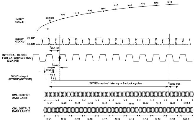
Figure 5. SYNC~ ACTIVE Timing Diagram
